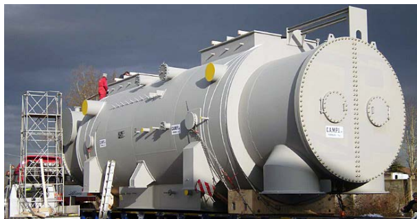
Figure 20: Steam Condenser (Courtesy: C.A.M.P.I.)
