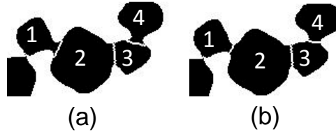
Figure 2.4: The comparison of two watershed segmentations: (a) the result of the original UECS; (b) the result of the revised UECS with a timed erosion-dilation process.
