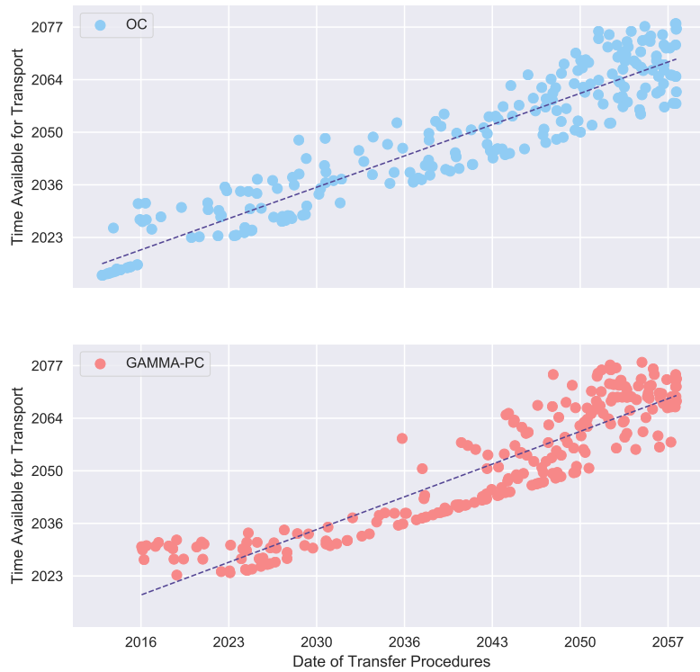
Figure 4.14: Scatter plots comparing the transportation eligibility dates of an OC solution with the recommended GAMMA-PC solution for the Comanche Peak loading problem (MPC-32).
