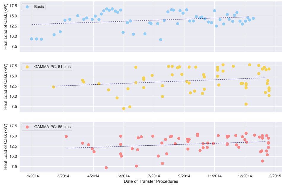
Figure 4.29: Scatter plots comparing the initial cask heat loads for the recommended Zion loading plan and its alternate to the basis solution over the original timeline.
