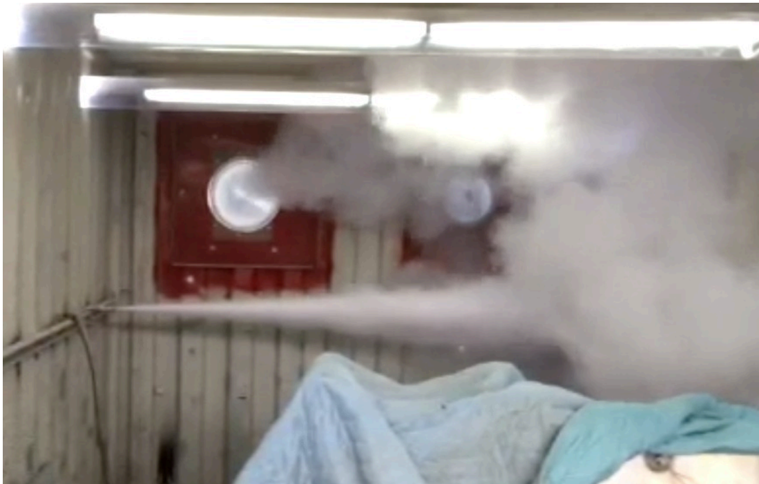
Figure 21 - Fire extinguisher test fire.
