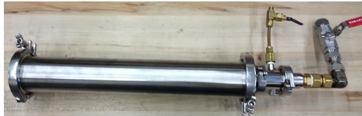
Figure 33 - Produced Gas Condenser
