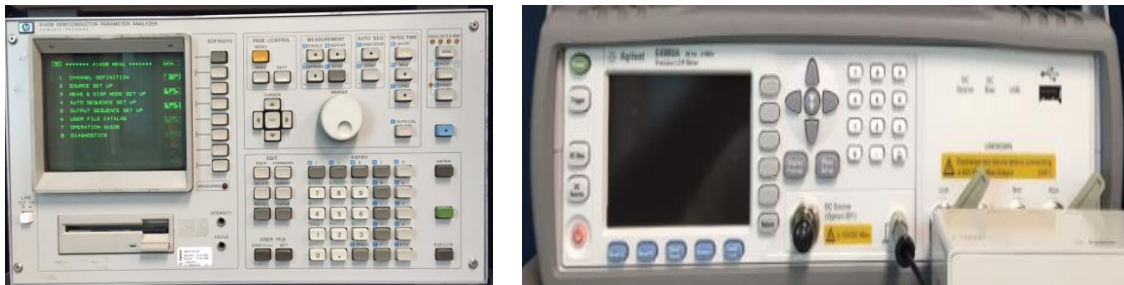
Figure 20 HP 4145B and LCR 4980 Meter used for electrical analysis [picture from research lab]
