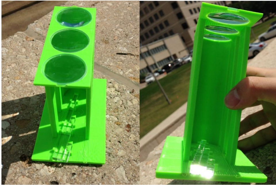
Figure 57. The demonstration of 1 \times 3 lens-to-channel waveguiding concentrator system.
