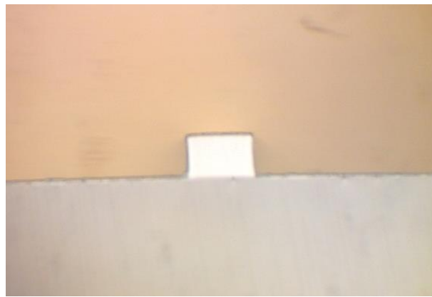
Figure 47. Photograph of the cross section of the polished SU-8.
