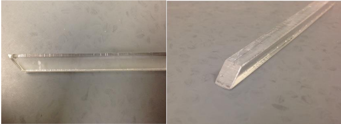
Figure 53. A PMMA waveguide is made by CO2 laser cutter.
