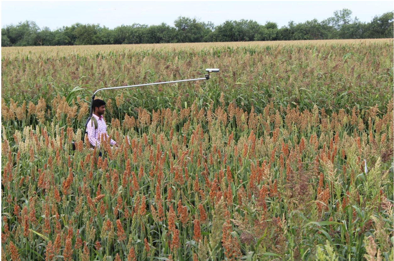
Figure 2.1. Backpack-sensing frame with ACS-430 crop circle sensor mounted on top to collect NDVI data.
