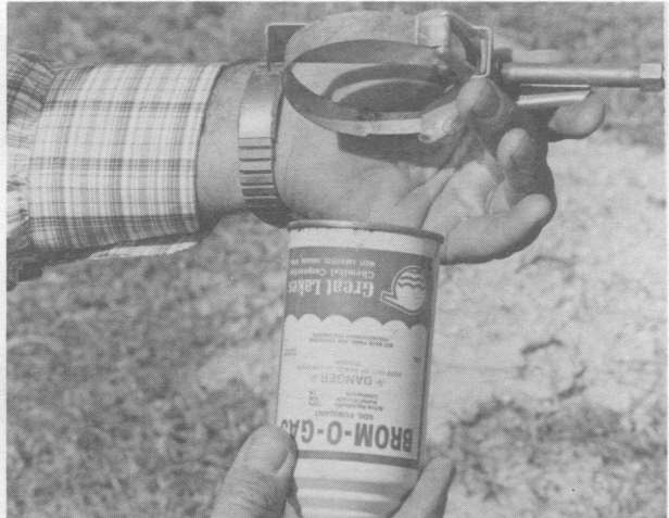
10. Hold the container of gas upside down and place the applicator on the bottom of the can.
