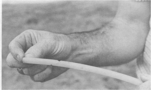
8. Notches may be cut in the side of tubing (approximately 1-1½" from end) to allow gas to escape into hole should tubing become plugged with soil.
