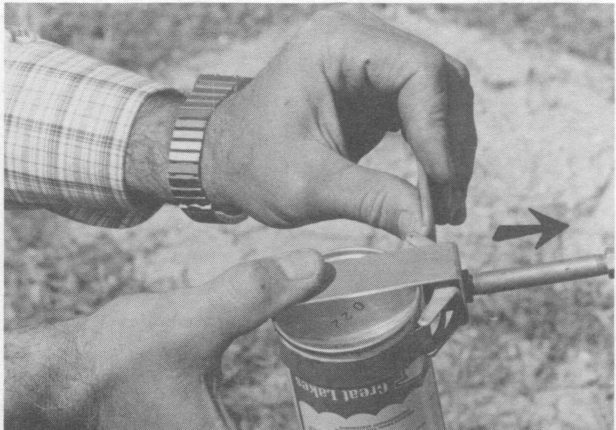
12. Hold the can upside down with the nozzle tip or outlet pipe directed away from the body, as indicated by the arrow. Carefully pull the lever backward, allowing the metal tubing to penetrate the can.
