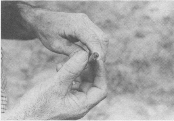
7. Tube may become plugged if forced into the soil. This should be avoided.
