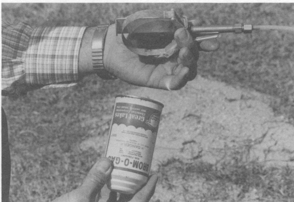
15. Once can is empty, pull latch forward. This allows the can to fall from the applicator.
