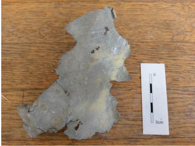
Figure A.9- CAMP-4701 is a piece of skin from a WWII P-47 aircraft found on a beach in North Carolina, recovered, then stored outside. Photo by the author.
