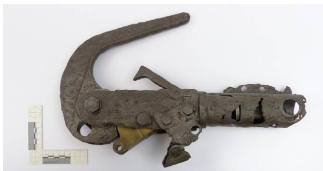
Figure J.6- A 'skyhook' recovered from Biplane 3 in Field A. It was conserved at ECU soon after recovery. This artifact is at the National Naval Aviation Museum. Photo by the author.
