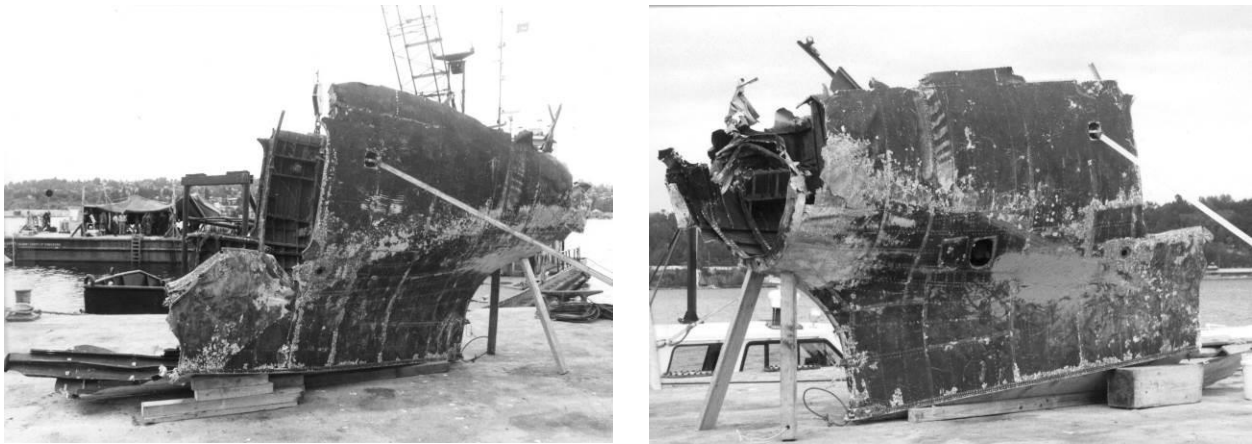
Figure 9.11- The recovered tail section of PBM-5 59172 (both side views) photographed on land in 1996 to show the areas of localized corrosion. The bottom part of the aircraft in the photo would have been exposed and the top part buried. The corrosion pattern shows the sediment line. Photos courtesy of NHHC UAB.
