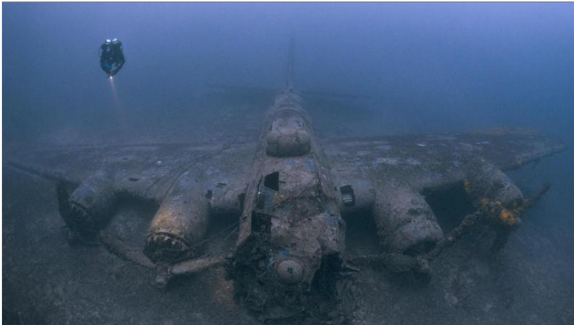
Figure 3.2b - A WWII B-17 wreck in 72 m off Vis, Croatia. The aircraft successfully ditched- damage to the nose is a combination of flak, possible bottom impact, and corrosion damage. Photo reprinted from Underwater 360 2018.
