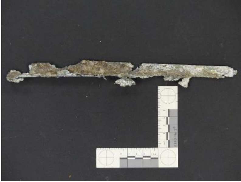
Figure 5.4- Sample RAFMDo01 is a fragile piece of stringer material that is pitting and exfoliating extensively. Photo by the author.
