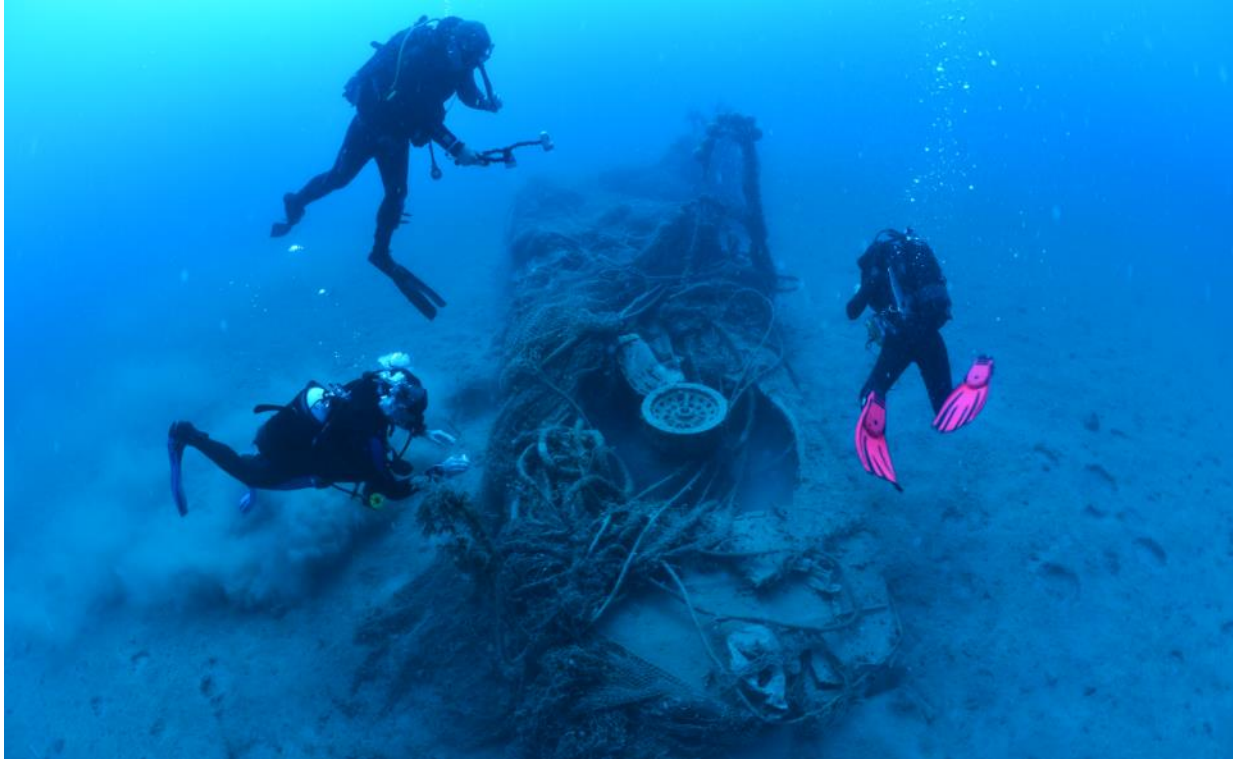
Figure 7.35- This B-24 wing lies close to the shore in the harbor of Komiza at 31 m deep. It was difficult to visually survey this wing as it is almost completely covered in netting. This starboard wing is missing both the leading and trailing edges, the tire, and the engines. Our team, the author on the right, is taking images for a 3D model and performing the corrosion potential analysis. Photo by Danijel Frka.
