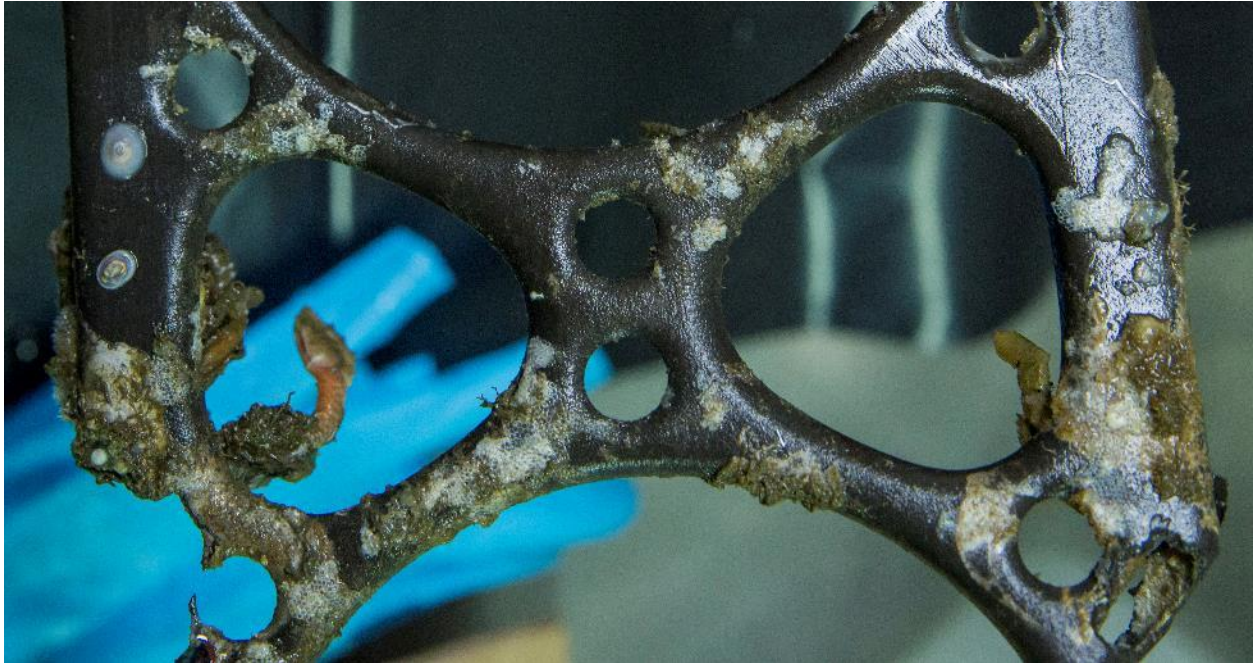
Figure 8.44- A sample of marine growth on the recovered frame piece. Also note the dark brown color of the metal surface. Photo courtesy of Juyle Newlin, OET.
