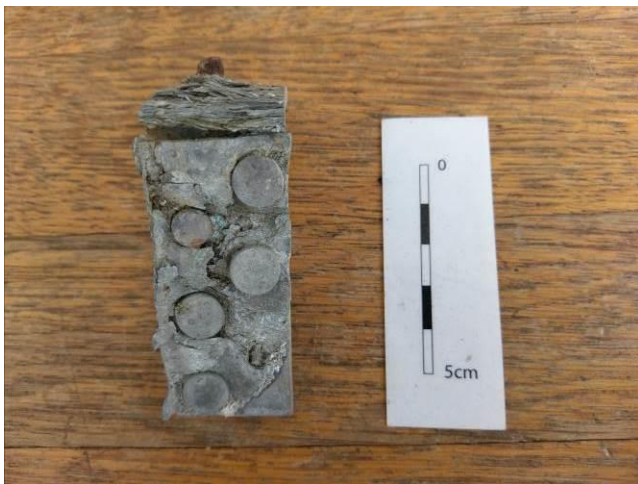
Figure A.10- CAMP-4702 is a piece of cast aluminum and rivets suffering from exfoliation corrosion. Photo by the author.
