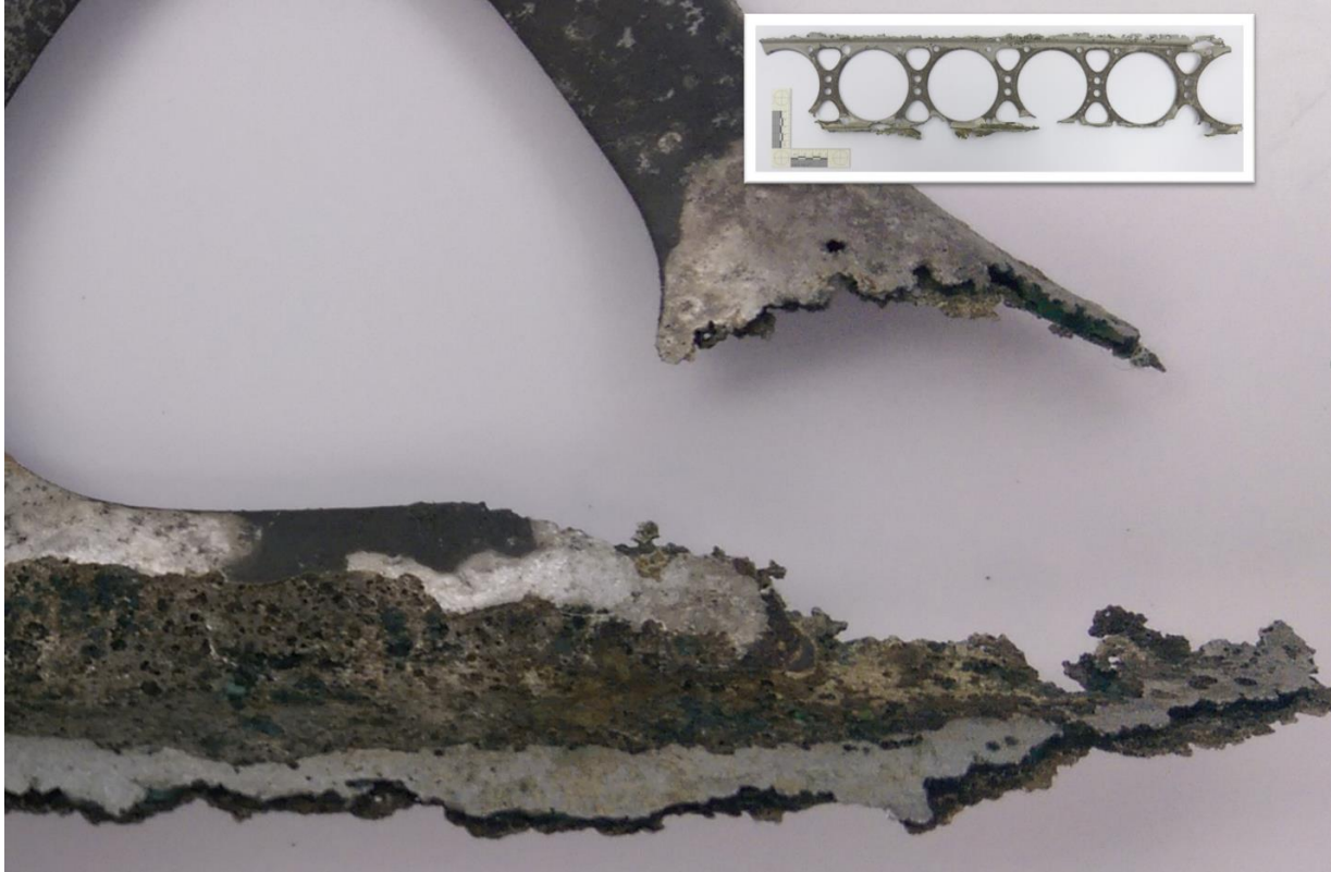
Figure 8.36- In this image the telltale brown microcrystalline wax indicated ER treatment common to iron artifacts at the time. The piece is currently also displaying green copper corrosion products, signaling continued pitting. Photo and inset by the author.
