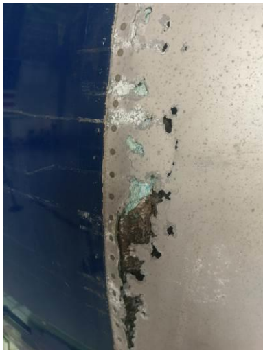
Figure 5.2- An interesting set of corrosion products appear on the two GE CFM56-5B4/P turbofan engines of the 'Flight 1549' Airbus A320-214 aircraft that crashed in the Hudson River in 2009. These engines were only submerged for a few days in brackish water, but did not undergo any conservation treatment and have consequently developed a range of issues. These engines will be treated in 2019 by a team of archaeologists, conservation specialists, museum professionals, and airline maintenance professionals. Photos by author with permission from the Carolinas Aviation Museum.
