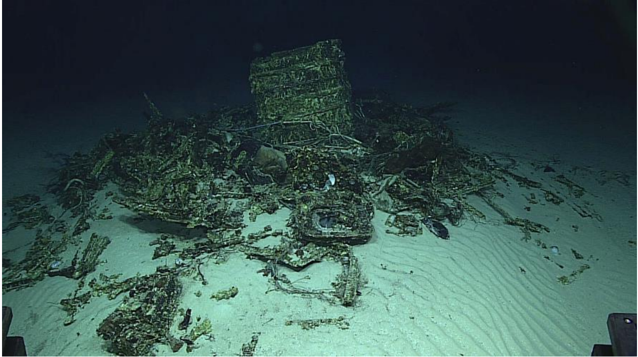
Figure 4.6- Remains of the top turret and the navigator's instrument panel and window. Photo courtesy of NOAA Office of Ocean Exploration and Research, 2016 Deepwater Exploration of the Marianas.
