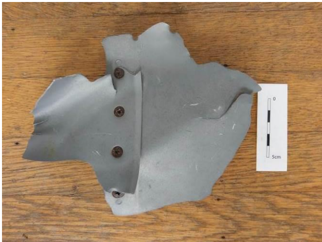
Figure A.6- A recovered piece of T-33 aircraft skin from a terrestrial crash site in Greenland. T-33 is post-WWII era, one of the first jet aircraft. Photo by the author.
