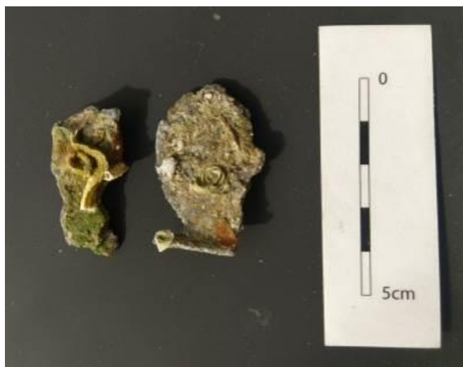
Figure A.1 - There are multiple aircraft wrecks around Vis island, off the coast of Croatia. Along with fieldwork on The Tulsamerican site, I visited dump sites for aircraft debris in local harbors. I took sediment, water chemistry, and corrosion potential readings from two of the dumped B-24 wings in 2015. I discovered small metal fragments in one of the sediment samples, VISB-2401 and VISB-2402, and decided to analyze these fragments with XRF. VISB-2401 (R) and VISB-2402 (L) are possible aluminum samples. Both present with a large amount of biofilm, some calcareous encrustation, and other marine growth. Upon scraping, VISB-2401 clearly is shiny bright metal, while VISB-2402 remains a dark color and resembles lead. Photo by the author.
