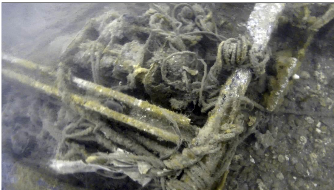
Figure 3.2g - Netting and rope wrapped around the structural interior of a B-17 wing in the English Channel. The shifting sands have scoured away the skin over time. Photo courtesy of The BentProp Project, Ltd.
