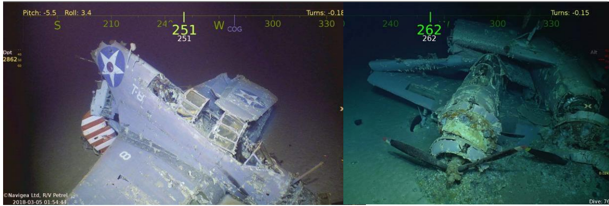
Figure 3.2c - Bright paint and organic covers on the flight control surfaces of this TBD Devastator remain remarkably intact (L). Aircraft from this site, the USS Lexington aircraft carrier, are all in similar condition and show deepwater preservation (2800m+). Note the comparatively accelerated deterioration of the engines (R) and the corrosion products fanning out from them on the sea floor. Photos reprinted from Paul Allen's website (The Editors 2018).
