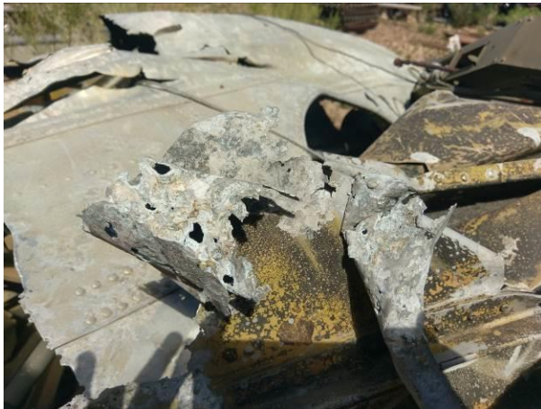
Figure 9.27- Areas of corrosion next to areas of intact and primer-covered metal on a piece of PBM-5 59172 aft fuselage (L), currently in outdoor storage at Pima Air & Space Museum. The vertical stabilizer's metal (R) is bleached but otherwise in good condition. Photo by the author (L) and Andrew Boehly (R).
