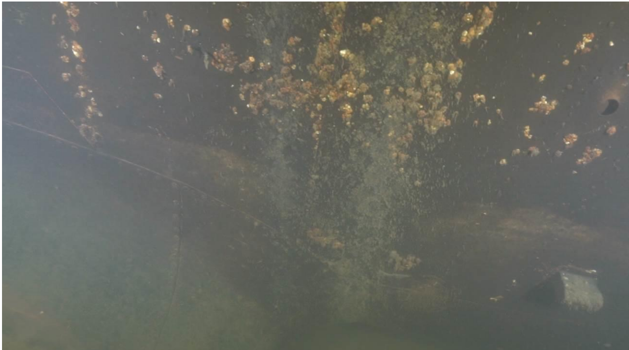
Figure 9.15- An area of algae growth on the fuselage in the path of released gas bubbles (brightness adjusted to show the growth). Photo by Kees Beemster Leverentz.
