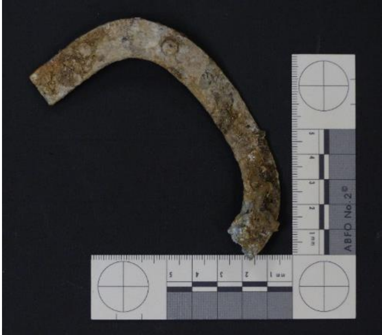
Figure 5.6- RAFMD03 is a cast aluminum curved object with four aluminum rivets and one ferrous rivet. The ferrous rivet is surrounded with rust. The object was painted with a light blue paint and remnants of it remain on the surface along with dirt. Photo by the author.
