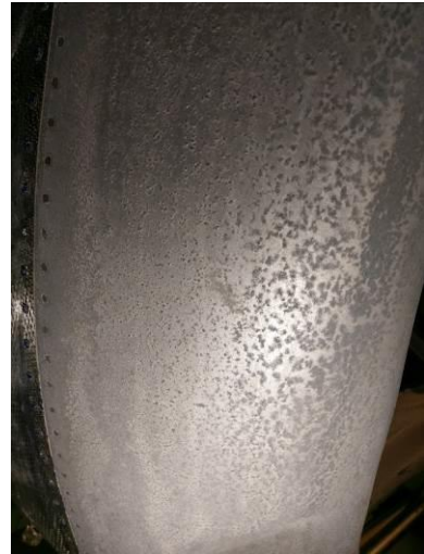
Figure 5.2- An interesting set of corrosion products appear on the two GE CFM56-5B4/P turbofan engines of the 'Flight 1549' Airbus A320-214 aircraft that crashed in the Hudson River in 2009. These engines were only submerged for a few days in brackish water, but did not undergo any conservation treatment and have consequently developed a range of issues. These engines will be treated in 2019 by a team of archaeologists, conservation specialists, museum professionals, and airline maintenance professionals. Photos by author with permission from the Carolinas Aviation Museum.
