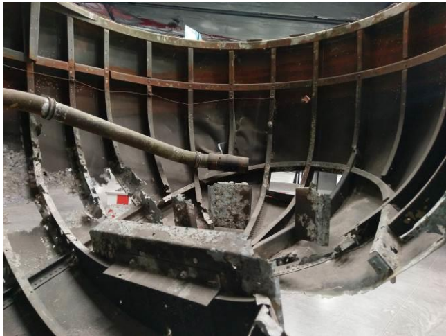
Figure N.1 – PBM-5 recovered tail section showing areas of damage and corrosion. Likely the loss of the panel was due in part to the corrosion of the stringers underneath. Photo by the author.
