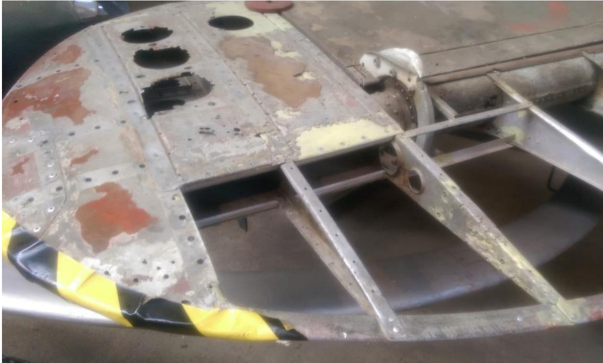
Figure 5.13- This Wellington bomber was recovered from Loch Ness in 1985 and is on display in Brooklands Aviation Museum, UK. It has been restored by placing compromised material on top of new material to retain the original shape. Burgess notes: “in this example, a middle ground was found between the competing demands of archaeology, which requires material to be kept in an ‘as is’ condition, and those of aircraft enthusiasts who wish to reconstruct aircraft to an ‘as new’ condition.” 191 Photo by the author.
