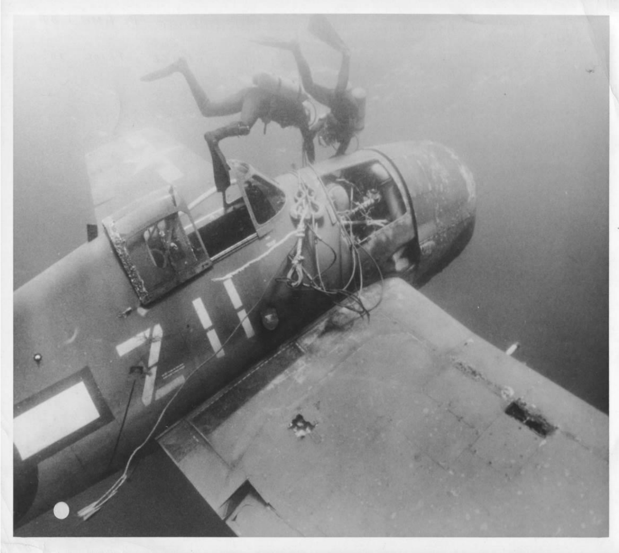
Figure 2.13- Divers rig F6F-3 Hellcat BuNo 66237 for lifting. Reprinted from Stafford 2008.
