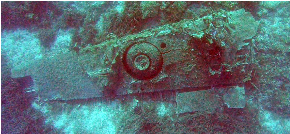
Figure 7.34- This B-24 starboard wing is located in a shallow bay on the northwest side of Vis at 14 m. It presents visually as intact except for either wreckage or drag damage, with almost no pitting loss or encrustation and only a thin layer of marine growth. Photo by Dr. Bridget Buxton.
