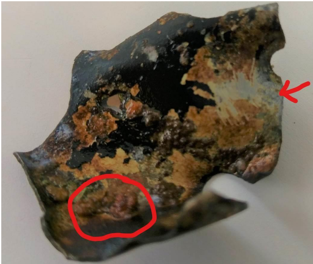
Figure 9.19- (Top) Side B of the PBM-5 sample after scraping a nodule of corrosion, which shows to be pitting through the wall of the piece from side A (bottom). The arrow on side A shows scraping of the tan color to reveal bare metal, showing loss of paint. Photos by the author.
