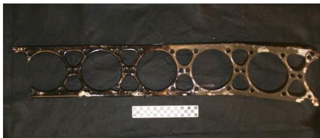
Figure J.11- A piece of girder frame, recovered in 2015. This piece has undergone conservation and is currently at the NHHC UAB lab. Photo by the author.
