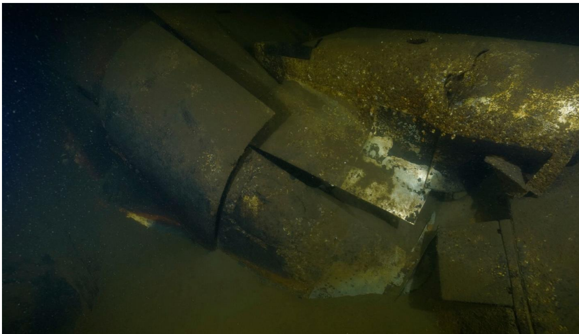
Figure 9.17- The starboard side engine with aluminum and stainless steel panels. Photo by Kees Beemster Leverentz.
