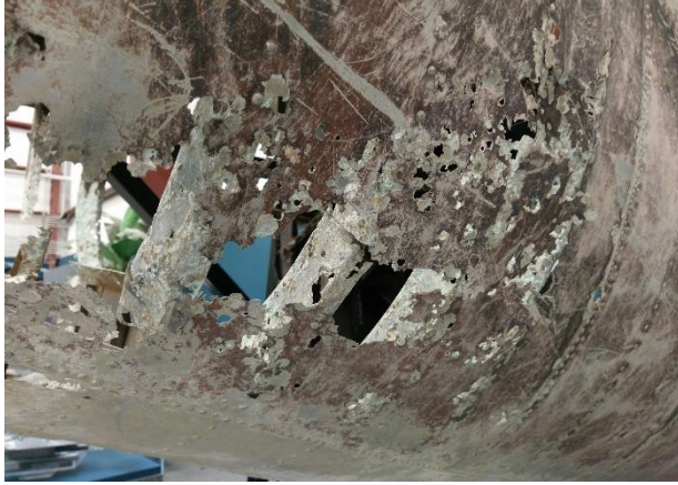
Figure 9.26- Areas of the PBM-5 59172 tail, currently on indoor display at Pima Air & Space Museum. Notice the extensive corrosion on the left photo, compared with the photo on the right, where an area shows primer and faded paint, as well as patches of bare metal. Photos by the author.
