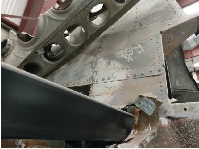
Figure N.3- An exterior view of the tail section showing some faded paint lines. Bare metal interior structure pieces show little corrosion. Photo by the author.
