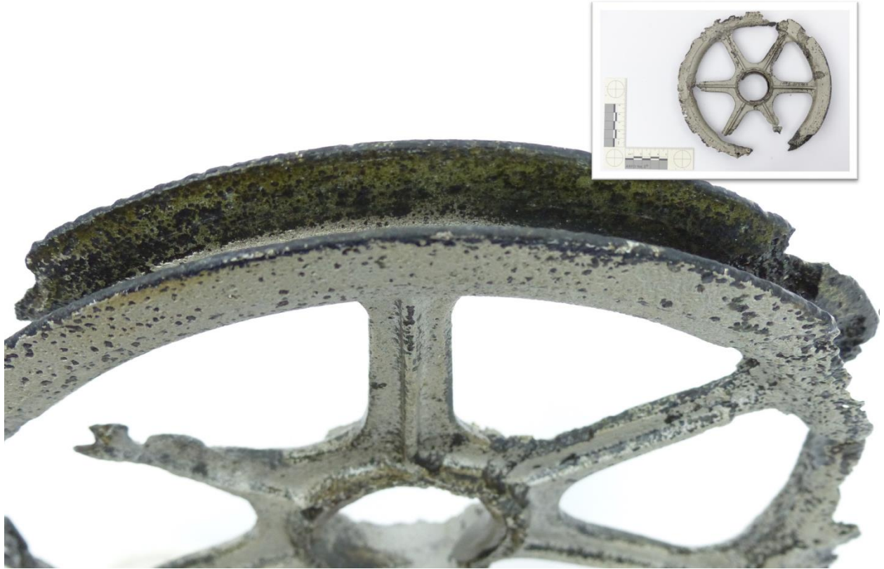
Figure 8.34- This piece of cast aluminum, recovered from the Macon wreck in 1991 and conserved by ECU as well, displays the brown wax no continued corrosion. Photo and inset by the author.
