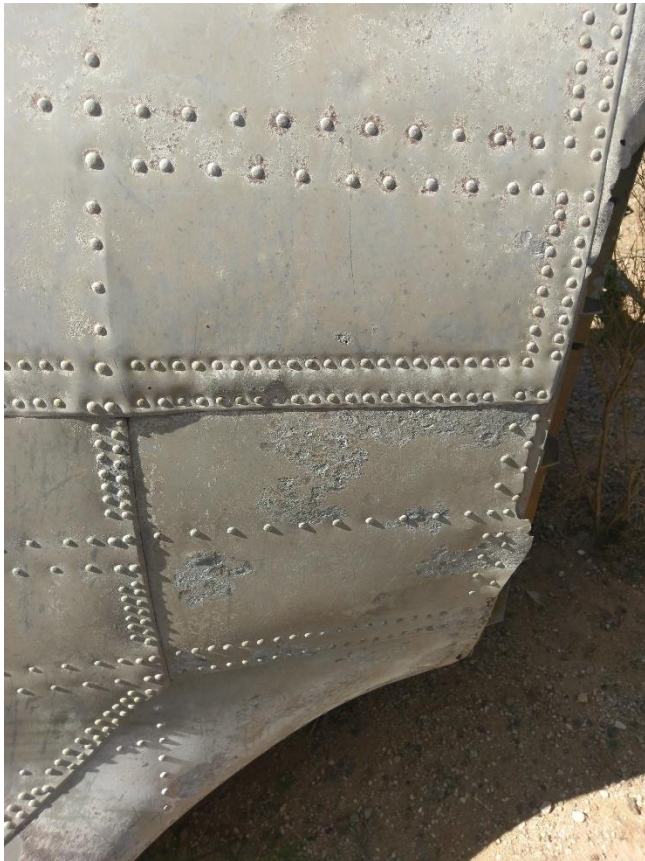
Figure N.14- Light corrosion patches on the rear afterbody of PBM-5 59172, resting on its side in outdoor storage at Pima Air & Space Museum. Photo by the author.
