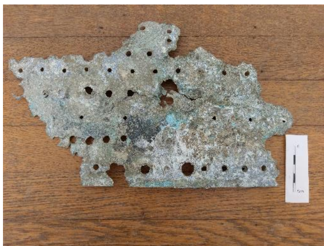
Figure A.4- A sample from the Norsk Luftfartsmuseum from a Focke Wulf 190 aircraft, WWII-era. This sample NLMFW-19001 was recovered from the ocean surrounding Norway and left exposed to the environment. Photo by the author.
