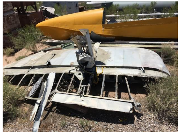
Figure 9.27- Areas of corrosion next to areas of intact and primer-covered metal on a piece of PBM-5 59172 aft fuselage (L), currently in outdoor storage at Pima Air & Space Museum. The vertical stabilizer's metal (R) is bleached but otherwise in good condition. Photo by the author (L) and Andrew Boehly (R).
