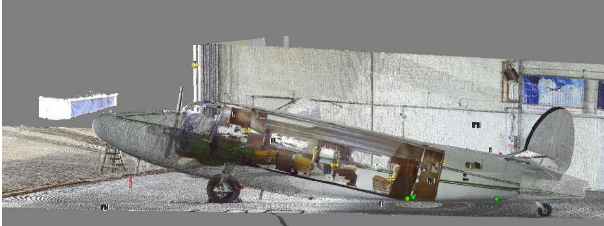
Figure 2.11- A 3D scan of the interior and exterior of a Lockheed Lodestar at The 1940 Air Terminal Museum in Houston, TX. Model by R. Warden, assisted by L. Champagne and the author.
