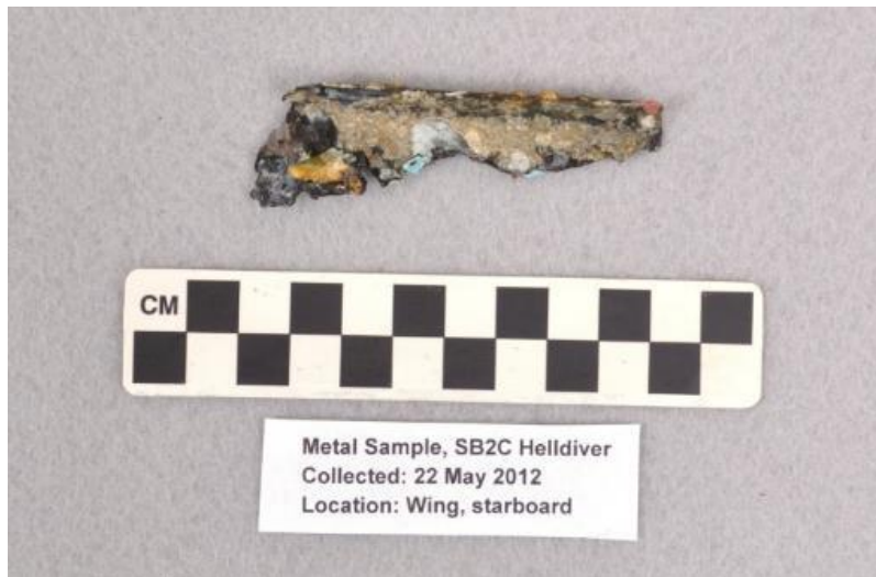
Figure 5.7- UABSB2C01 aluminum sample outward side. It appears that the outwards angled side of the metal sample is plated with a thin layer of metal that is different from the structural metal; i.e. a laminate, or alclad. Photo courtesy Kate Morrand, NHHC UAB lead conservator.
