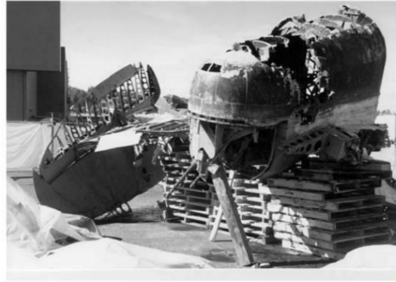
Complete Martin twin .50 cal tail turret less glass
