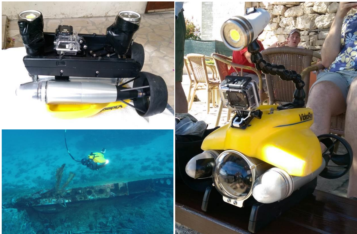
Figure 7.24- A VideoRay Pro4 ROV with GoPro cameras attached. Photos by the author.
