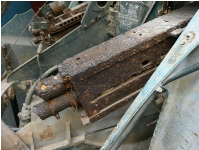
Figure N.6- One of the two M2 Browning machine guns inside the tail turret. Both display the same level of rusting and light pitting. Photo by the author.
