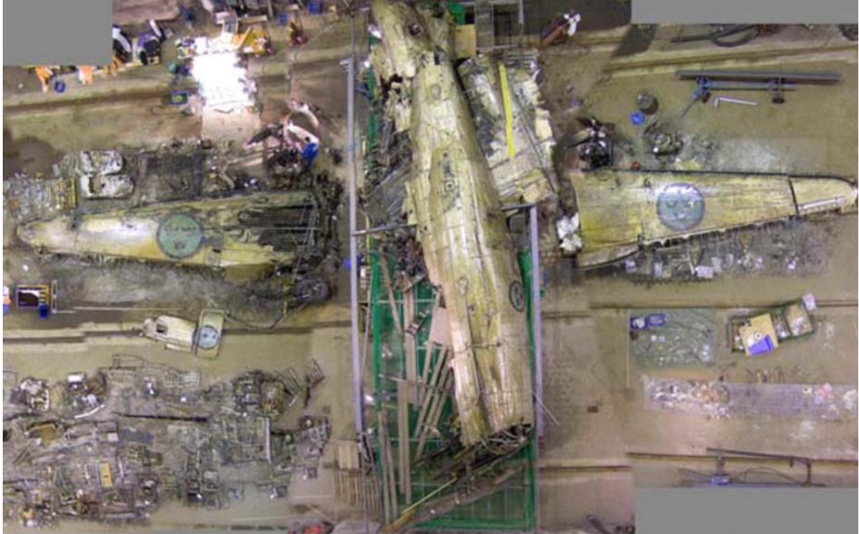
Figure 2.22- The DC-3 after it was raised and arranged for forensic study. Reprinted from LUTAB 2007.
