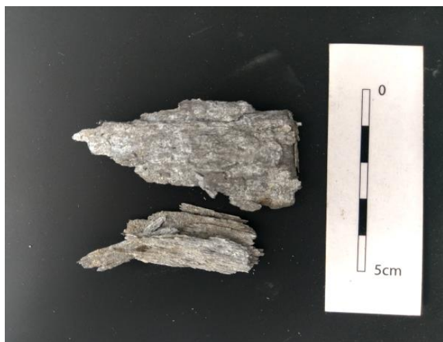
Figure A.2- RAFMDeH01 is a sample of propeller blade material from Handley Page Hampden that crashed in a terrestrial site in Russia in 1942 and was exposed to the elements until 1991. The sample was from the root of a propeller blade and had delaminated into thin slivers from exfoliation or intergranular corrosion. Photo by the author.
