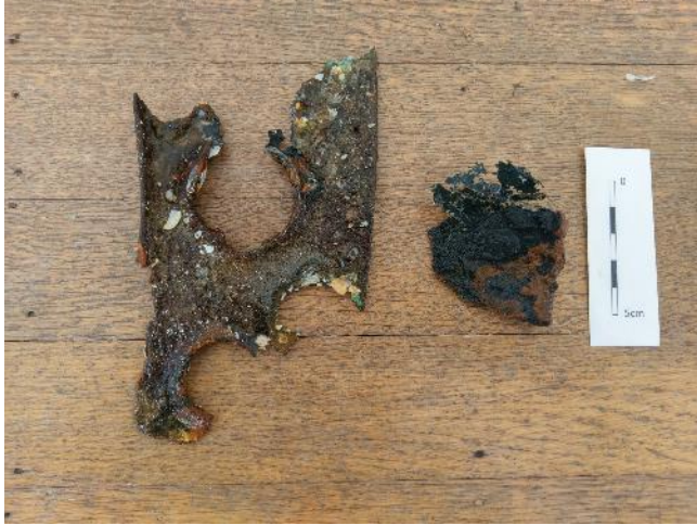
Figure A.7- Two samples from a WWII P-38 aircraft, submerged on a beach in Wales, UK. MoHP-3801 (L) is structural aluminum with a zinc-chromate primer, and MoHP-3802 (R) is, I believe, aluminum covered with corroded and concreted ferrous alloy metal from the engine. Photo by the author.
