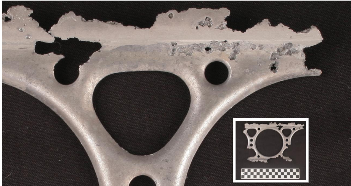
Figure 8.40- Frame piece USMPC01 after treatment to remove the powdery blue copper corrosion products, as seen in Figure 8.35. Photo and inset by the author.
