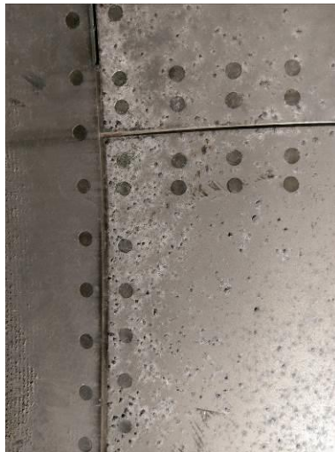
Figure 5.2- An interesting set of corrosion products appear on the two GE CFM56-5B4/P turbofan engines of the 'Flight 1549' Airbus A320-214 aircraft that crashed in the Hudson River in 2009. These engines were only submerged for a few days in brackish water, but did not undergo any conservation treatment and have consequently developed a range of issues. These engines will be treated in 2019 by a team of archaeologists, conservation specialists, museum professionals, and airline maintenance professionals. Photos by author with permission from the Carolinas Aviation Museum.
