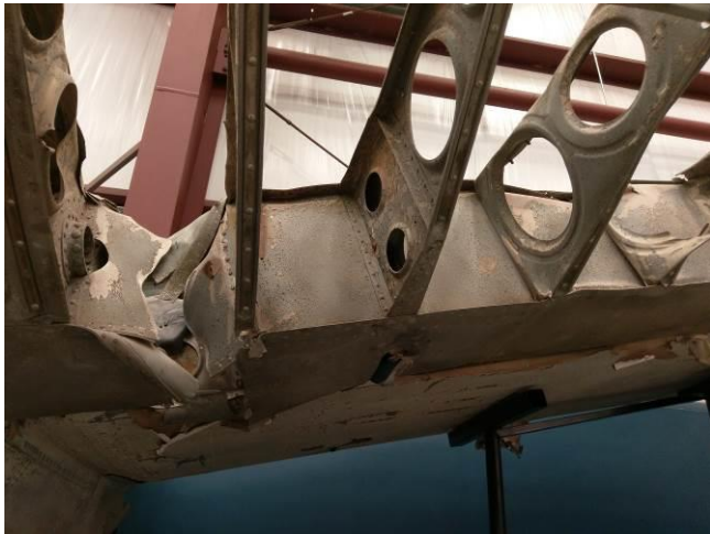
Figure N.4- Some chipping paint is still visible on the elevator structure. Photo by the author.
