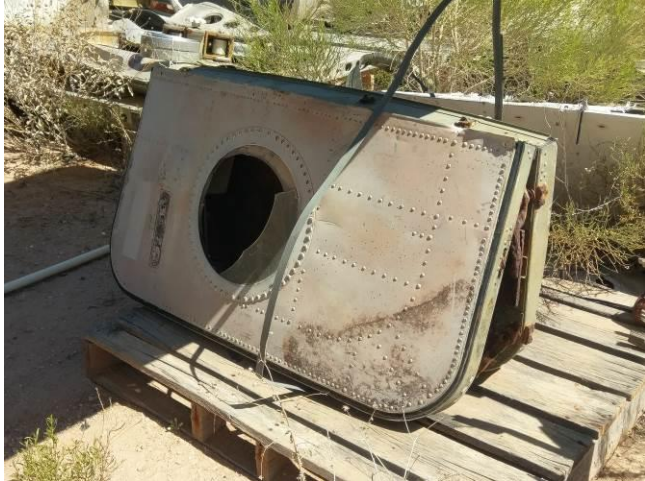
Figure N.13- An exterior tail section hatch door with mounts for jet-assisted take off (JATO) propulsion bottles, currently in outdoor storage at Pima Air & Space Museum. Photo by the author.
