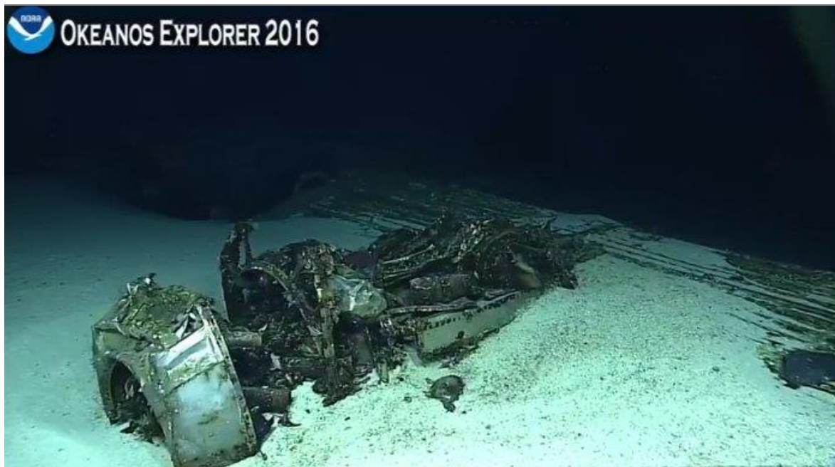
Figure 3.2d - An inverted WWII B-29 at 380 m found off Saipan. Shifting sands have worn away the exposed wing skin, showing the structure underneath. Note the scour pattern in front of the engine and the relatively excellent condition of the stainless steel cowling. Photo courtesy NOAA Office of Ocean Exploration.
