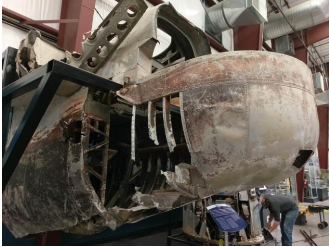
Figure N.1 – PBM-5 recovered tail section showing areas of damage and corrosion. Likely the loss of the panel was due in part to the corrosion of the stringers underneath. Photo by the author.
