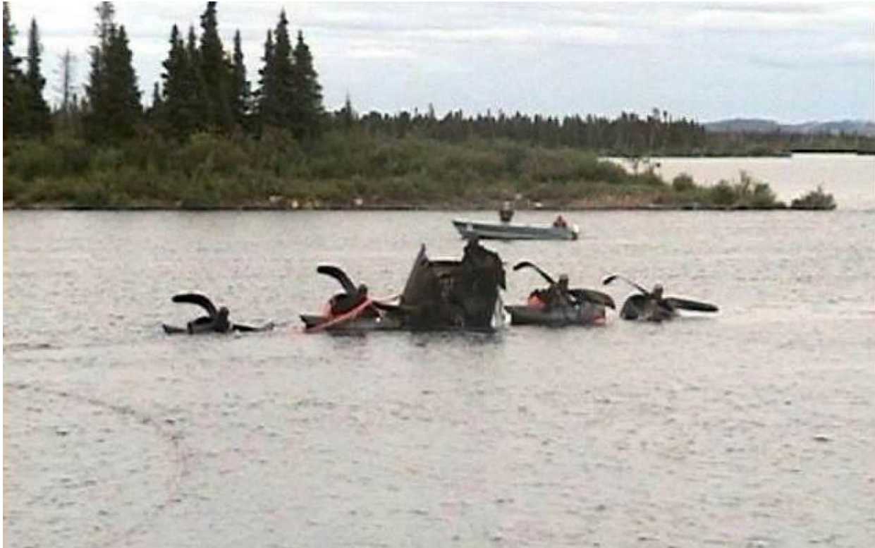
Figure 2.17- The B-17 as it first came to the surface supported by list bags. Reprinted from Skanes 2005.
