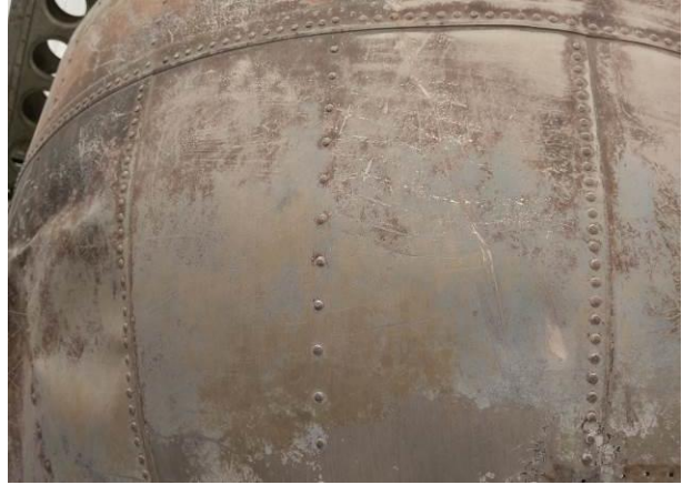
Figure 9.26- Areas of the PBM-5 59172 tail, currently on indoor display at Pima Air & Space Museum. Notice the extensive corrosion on the left photo, compared with the photo on the right, where an area shows primer and faded paint, as well as patches of bare metal. Photos by the author.
