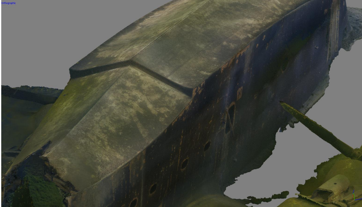
Figure 9.22- The curve of the hull and the step, beautifully rendered by Photoscan. Model by Kees Beemster Leverentz and the author.
