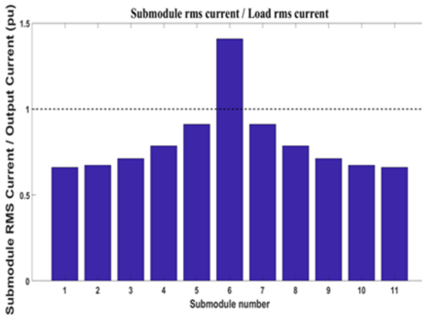
Fig. 31 Submodules current RMS rating as a function of the RMS output current in per unit for the 11 submodules design
