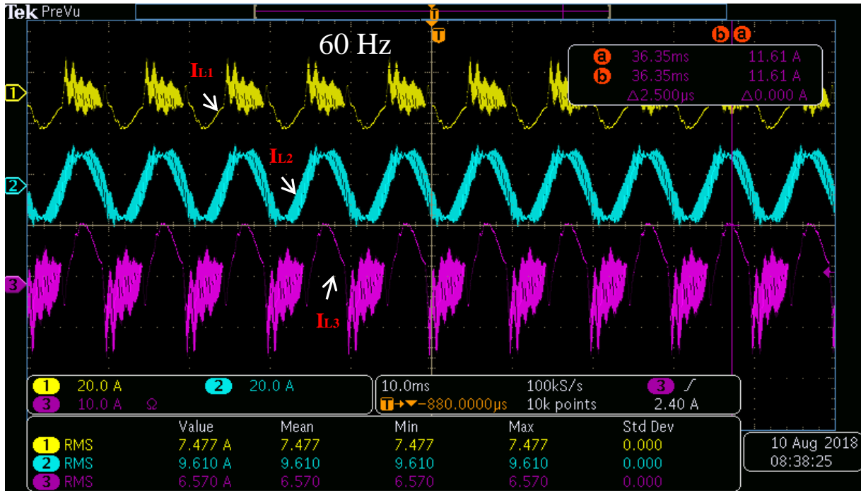
Fig. 71 The currents of the three inductors as seen in Fig. 27 when the output is 60 Hz. The ripple can be minimized by increasing inductor size or the switching frequency of the converter.
