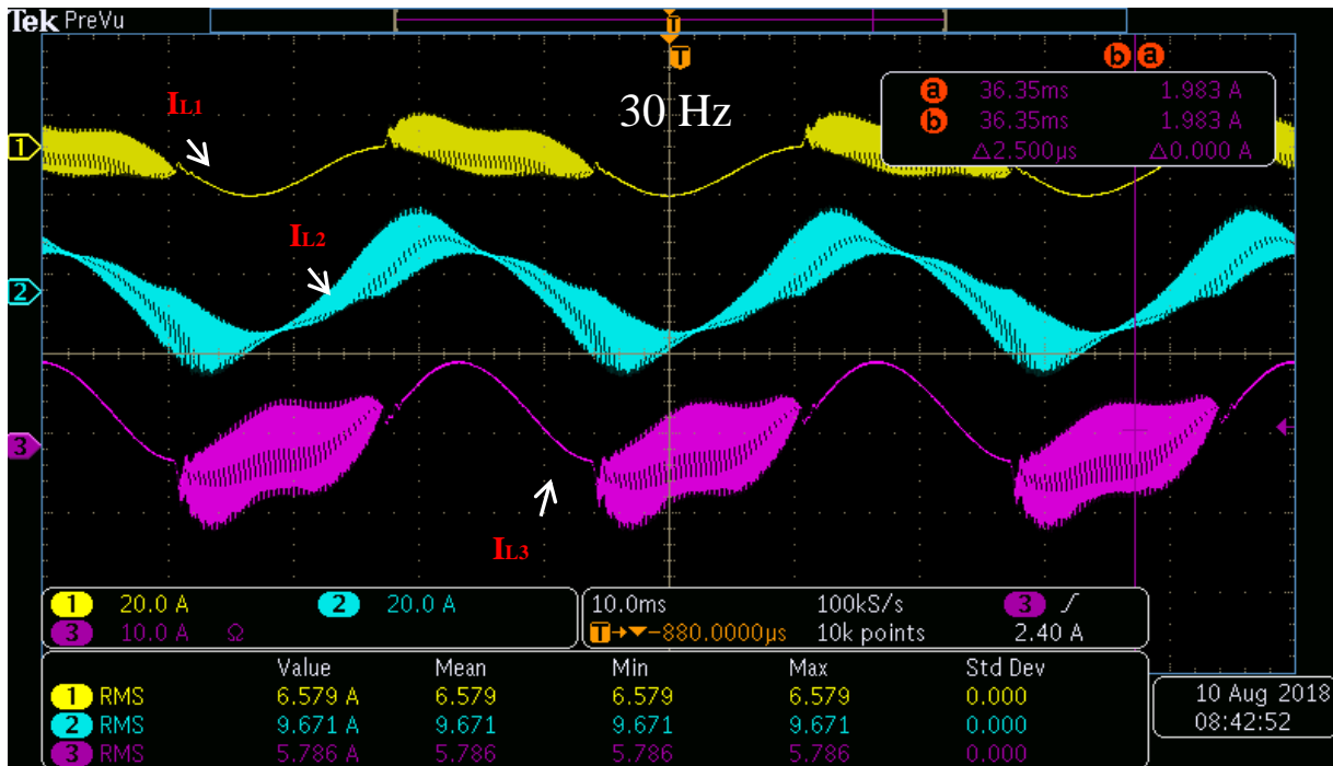
Fig. 72 The currents of the three inductors as seen in Fig. 27 when the output is 30 Hz. The ripple can be minimized by increasing inductor size or the switching frequency of the converter.
