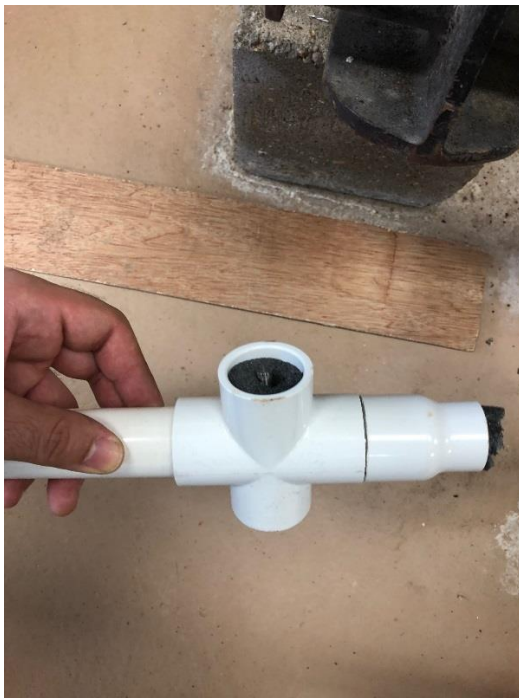
Figure 11: Distributed Sensing Array and PVC Centralizer
