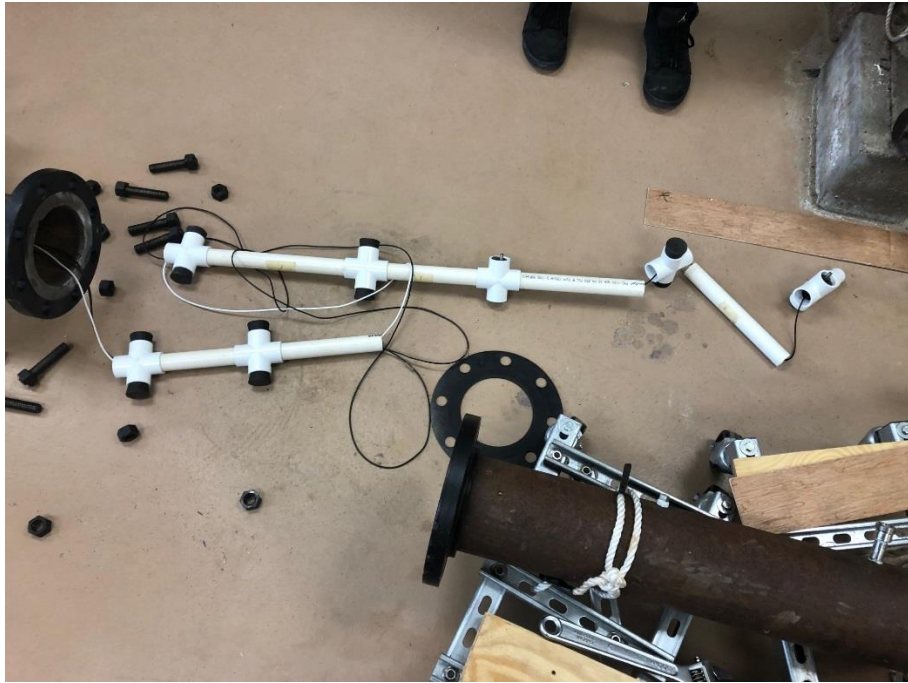
Figure 11: Distributed Sensing Array and PVC Centralizer
