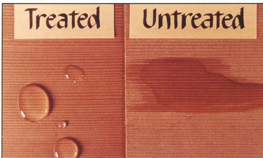
Wood that is treated with water repellent sheds water, but nontreated wood absorbs water quickly.
