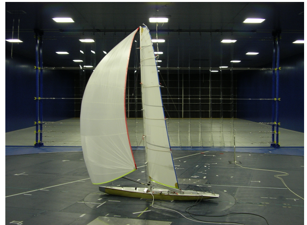
Figure 1: Photograph of the America's Cup Class 1:12.5 scaled model during the wind-tunnel test.
