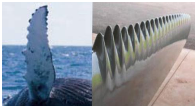
Figure 9.1 Humpback whale pectoral flippers, and Figure 9.2 Manufactured adapted tubercles on the leading edge of WhalePower wind turbine blade (Fish et al., 2011).
