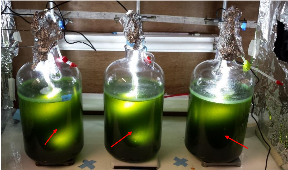
Figure 6.12 – Reactor set-up for the large-volume semi-continuous WWPA+C.v treatment with internalised LED strips. Red arrows denote dark zones. Image taken on day 4.
