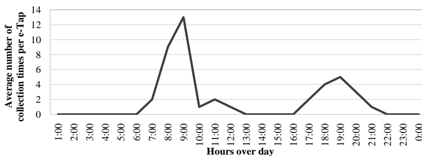
Figure 7. Hourly withdrawal variability of 28 e-Taps over one day in Jarreng.
