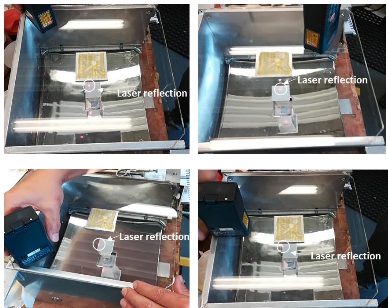
Figure 59. A photograph showing the laser beam reflection at the top of the homogeniser.
