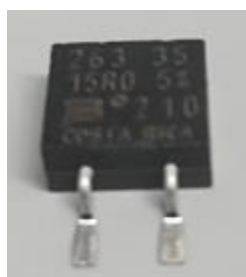
Figure 19. Photograph of electrical resistance heater (ERH).
