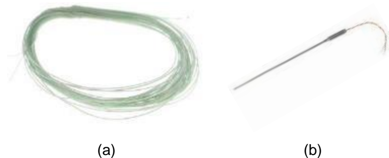
Figure 22. Photographs of K-type thermocouples (a) wire thermocouple and (b) pro type.
