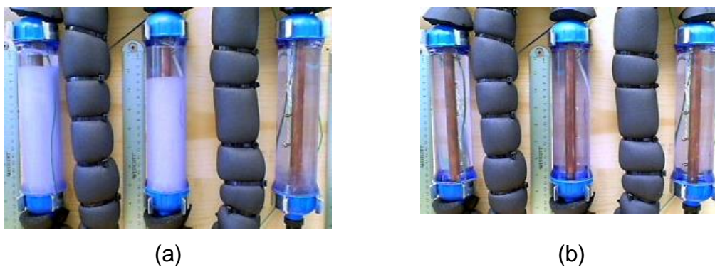
Figure 144. PCM melting photographs for case 2 (RT42-RT35-RT27) with HTF inlet temperature of 60°C and flow rate of 40ml/min at (a) 40min and (b) 240min.
