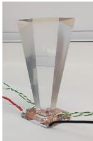
Figure 56. Photo of refractive homogeniser attached to the CPV assembly.
