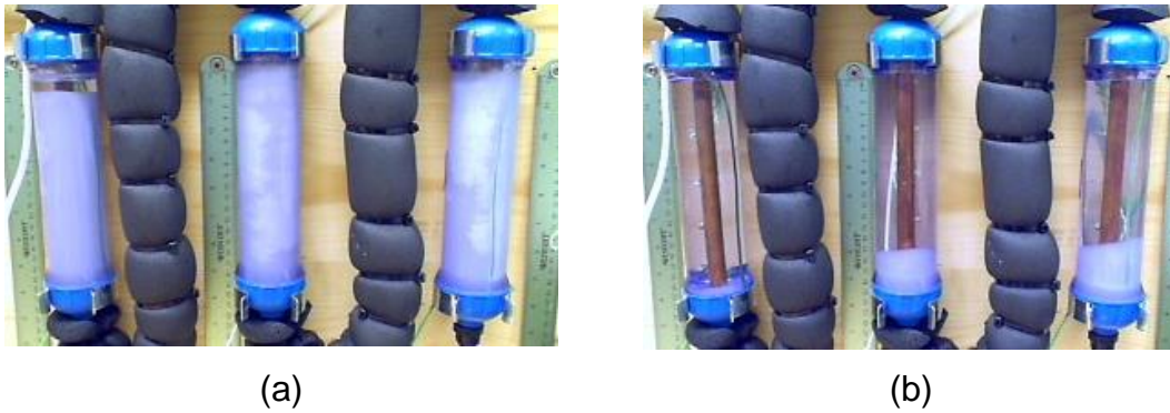
Figure 145. PCM melting photographs for case 3 (RT42) with HTF inlet temperature of 60°C and flow rate of 240ml/min (a) 60min and (b) 240min.
