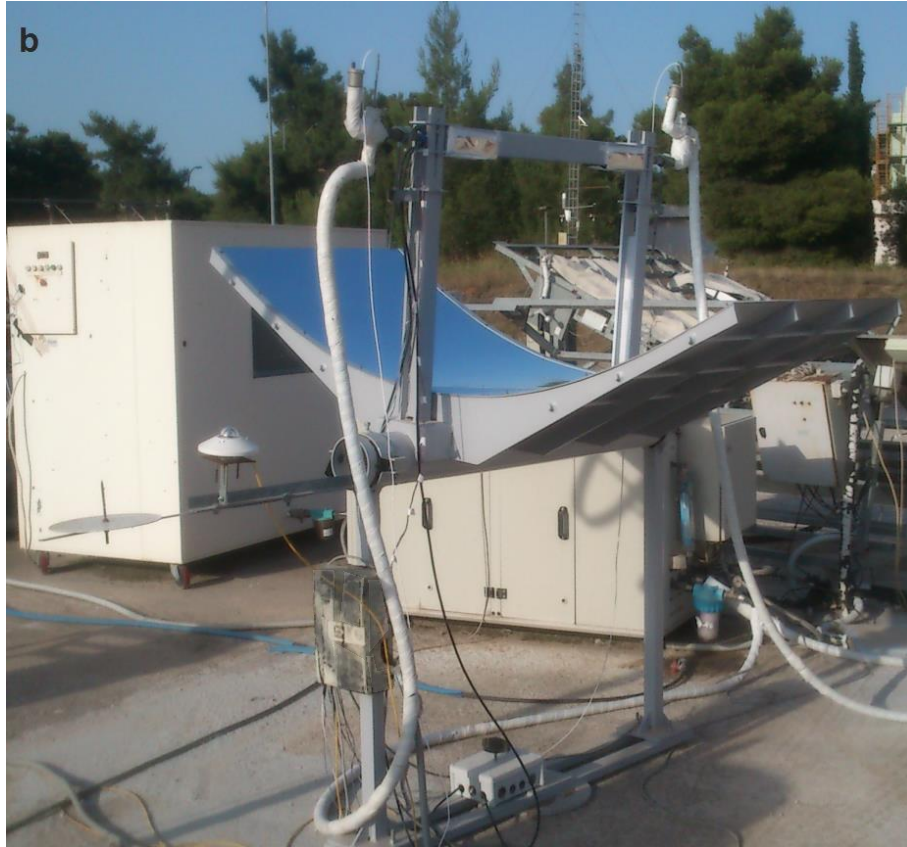
Fig. 1 Metallic structure of the CPVT system: (a) CAD drawing and (b) constructed frame.
