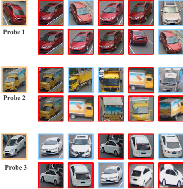
Fig. 4. Example vehicle re-identification results (rank-5) of two probes on the VeRI-776 dataset. For each probe, the first row correspond to the ranking results produced by our baseline, the second row describes the improved ranking results produced by our proposed method (GAN+LSRO+re-ranking). Vehicle surrounded by red box denotes the same vehicle as the probe, otherwise blue.
