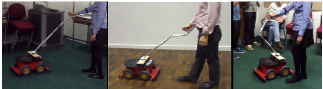
Figure 40, subjects following the robot with spring system in the handle fitted on a pioneer 3AT robot
