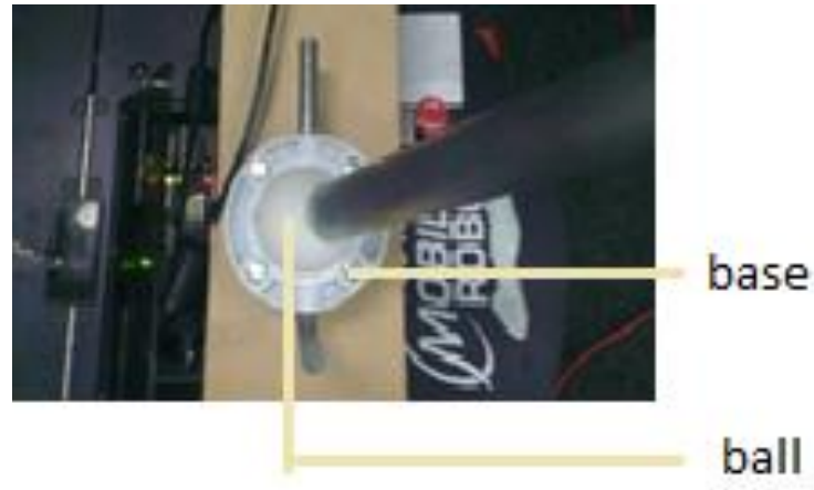
Figure 37, Ball-in-a-cup joint with detachable pin
