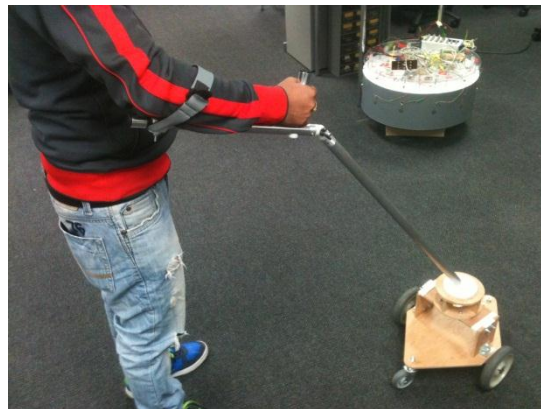
Figure 35, Crutch-Like design of the handle
