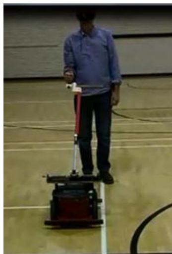
Figure 44, Handle mounted on the middle of the robot and attached to the handler
