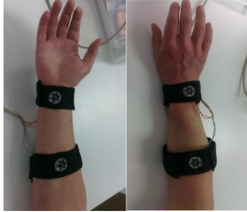
Figure 71, two sets of two vibration motors; left, attached to the inner side of the arm; right, attached to the outer side
