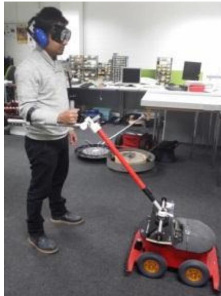
Figure 42, Handler attached to the handle with flexible joint
