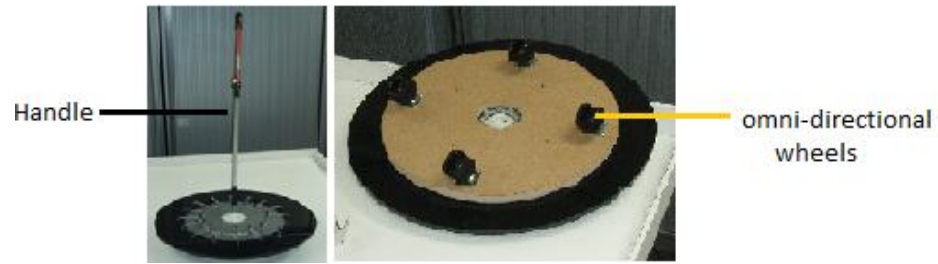
Figure 31, Robot-on-a-stick prototype with omni-directional wheels
