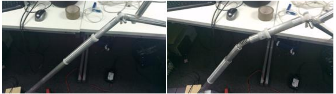
Figure 39, spring system in the handle
