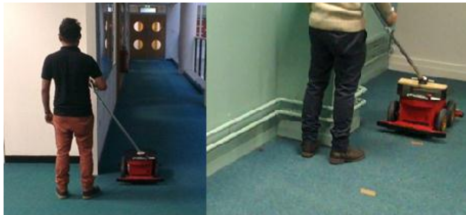
Figure 38, Handler losing track of the position of the robot with ball in a cup joint attached on a Pioneer 3AT robot
