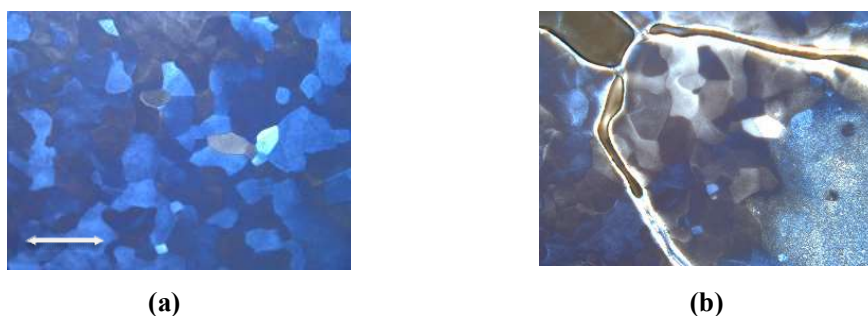
Figure 6.6: (a) Blue phase in an in-plane device (b) Degradation of polymer matrix on high voltage. Scale bar: 200µm.
