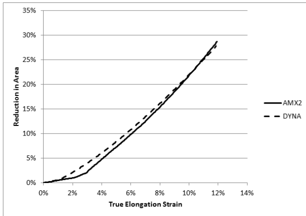
Fig. 10. Comparison of simulation and experiment for Reduction in area.
