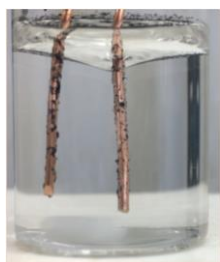
Fig. 1. Photographs of raw SWCNTs after 102 seconds electrolysis in DI water. The left electrode is the anode while the right electrode is the cathode.
