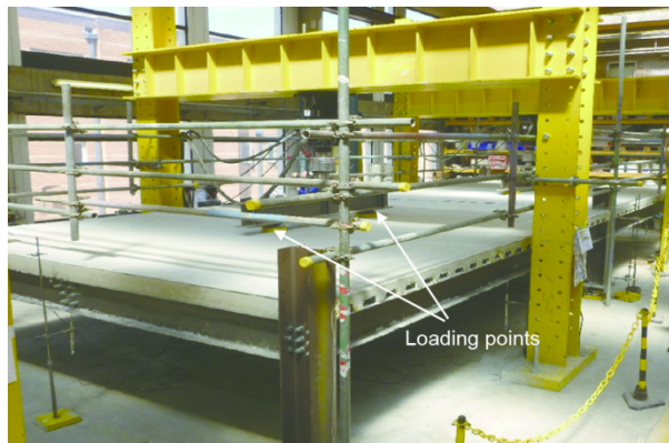
Fig. 11. Loads applied to the internal secondary beam.
