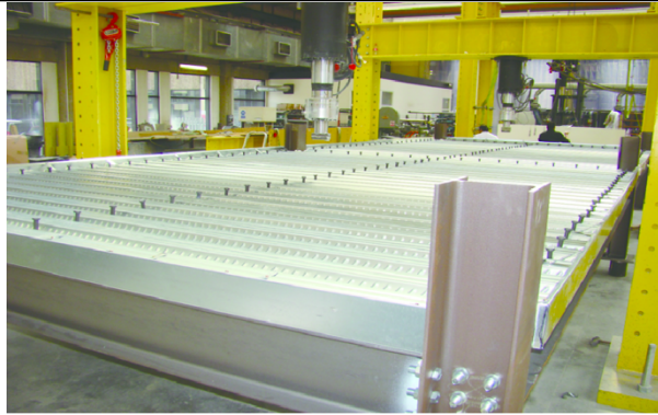
Fig. 4. Steel decking and shear connector arrangement.
