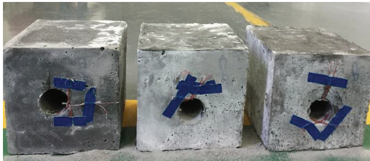
(a) Scaling tunnel model without reinforcement layer
