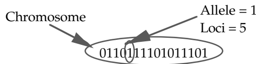
Figure 1 - An illustration of how a problem state can be represented as a string of numbers suitable for use within a GA.
