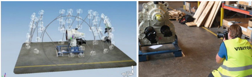
Fig. 2 In the Trial 2 Camera based photogrammetric 3D capture was applied in scanning a gear box at the OEM factory
