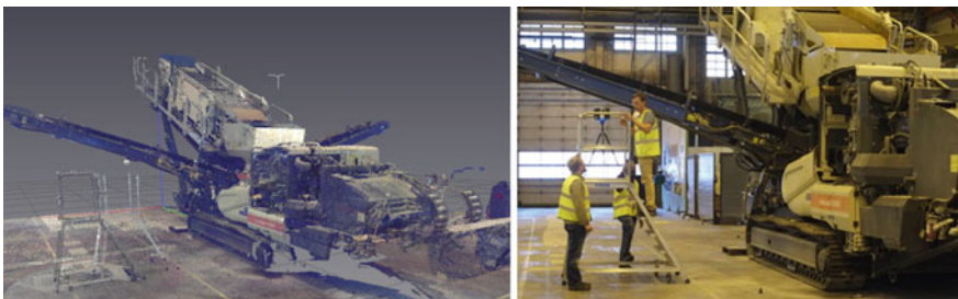
Fig. 3 Laser scanning and generated point cloud representation
