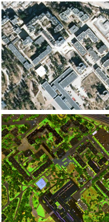
Figure 2. Comparison of an aerial ortho image and Titan intensity image in a 300 m × 300 m subarea. Ortho image © National Land Survey of Finland, 2013.
