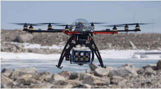
Figure 3: OktoKopter micro-UAV with 6-band multispectral sensor mounted on stabilised camera platform.
