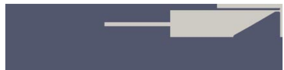
Fig. A-1 Geometry of the foot chamber of the Short Sg model with chamfers.
