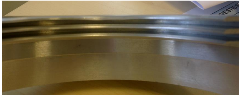
Oil deflector strain
