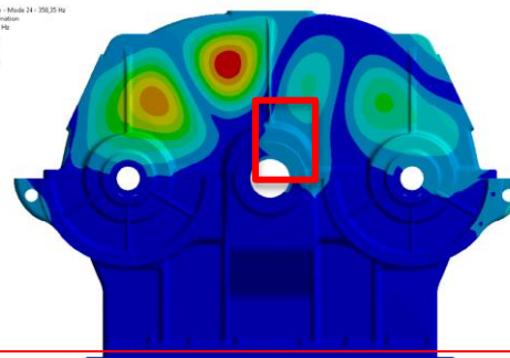
GB Casing- Modal analysis 350 Hz Mode shape (close to Pinion 1X)
