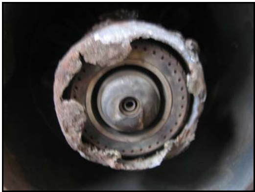
Figure 3. Fuel Injector Tip Sulfidation
