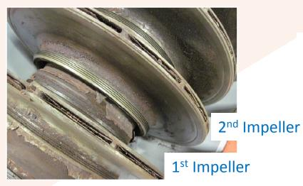
Fouling was most severe on 1<sup>st</sup> impeller and was progressively less to the 4<sup>th</sup> impeller.
