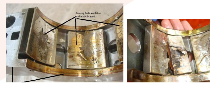
Journal bearings were subjected to very high cyclic load due to unbalance rotor after impeller breakage. Max bearing temperature recorded was 130°C.
