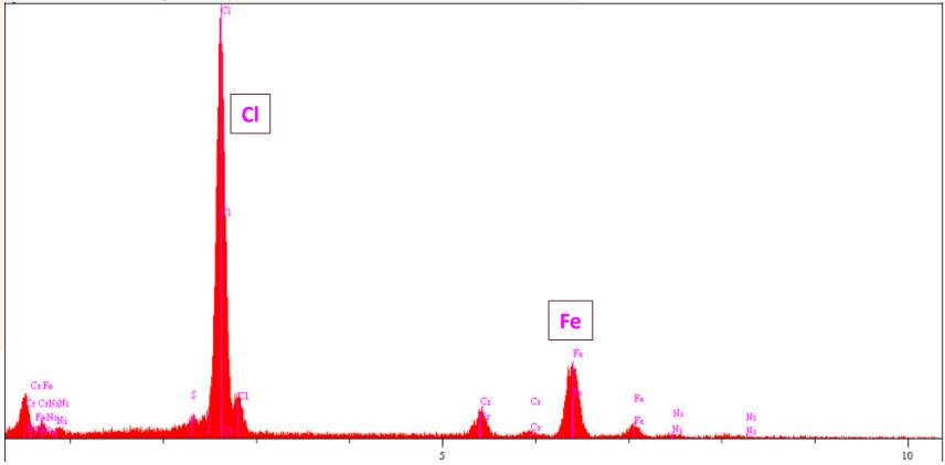
EDS Analysis of foulant on 1st Stage Impeller showing high Chlorides & Iron
