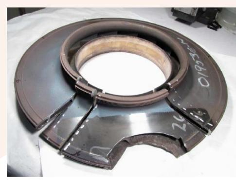
"The fracture surface is smooth, relatively featureless, and contains some evidence of beachmarks and thumbnails which are all characteristics of a fatigue failure".
