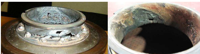
Figure 12: DLE Pre-chamber damage as the result of heavy hydrocarbon carry over and oxidation
