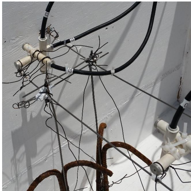
Figure 45 Specimen 3- Concrete Gage Arrangement
