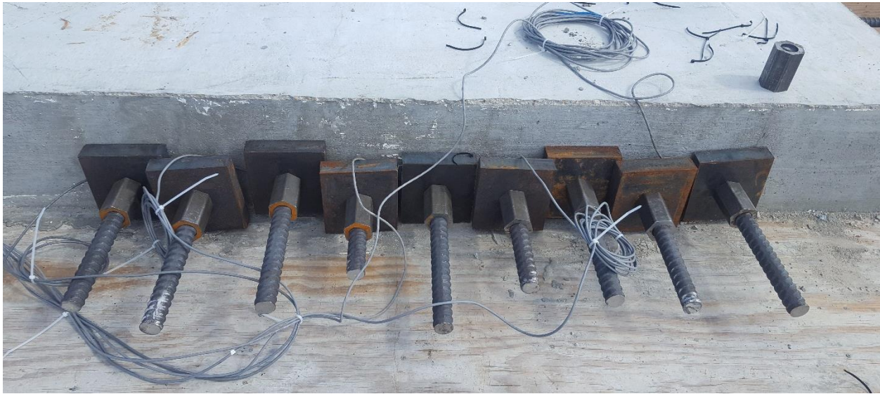
Figure 60 Specimen 1- Post-Tensioning Bars with Anchor Plates and Nuts, Side View
