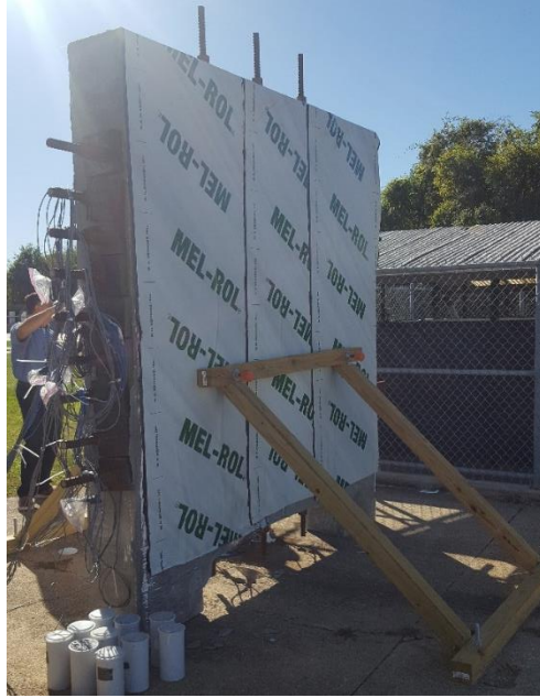
Figure 66 Specimen 1- Final Position with Weatherproofing Applied to One Side
