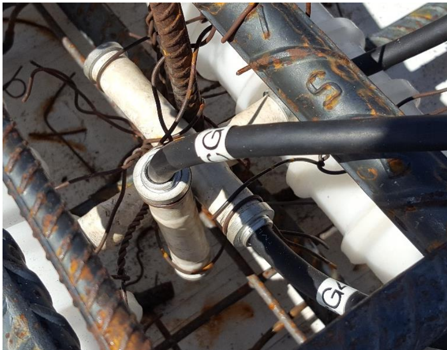
Figure 43 Specimen 1- Concrete Gage Arrangement
