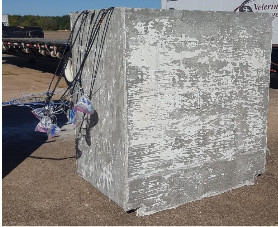
Figure 68 Specimen 3- Final Position (Weatherproofing Applied to Other Side)
