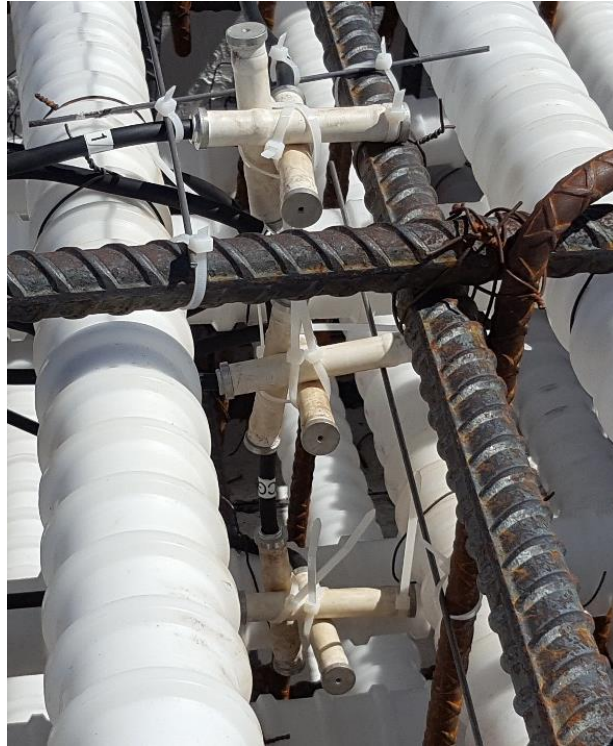
Figure 44 Specimen 2- Concrete Gage Arrangement
