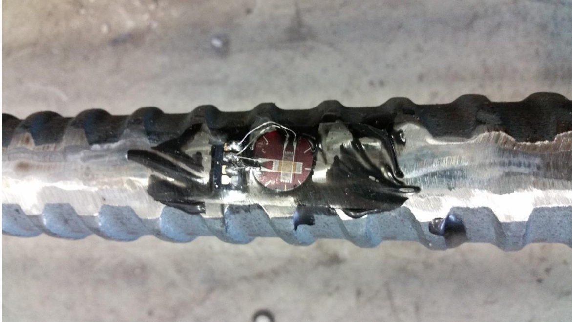
Figure 56 Post-Tensioning Bar with Strain Gage and Terminal Glued On
