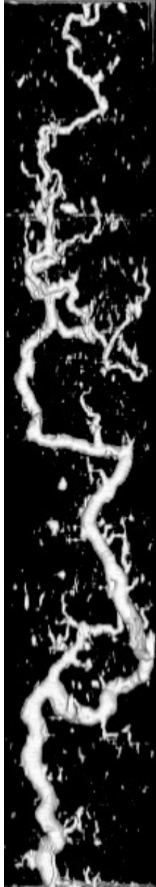
Figure 32. LDA16 wormhole structure
