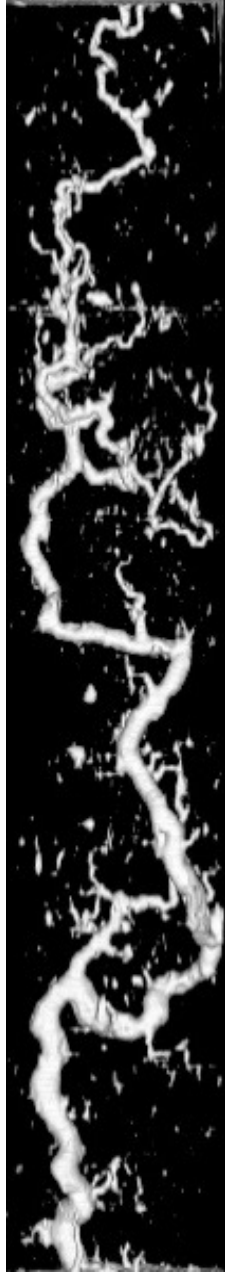
Figure A-65. CT Scan image of LDA16: v_i = 0.57 cm/min, PV_{BT} = 2.11
