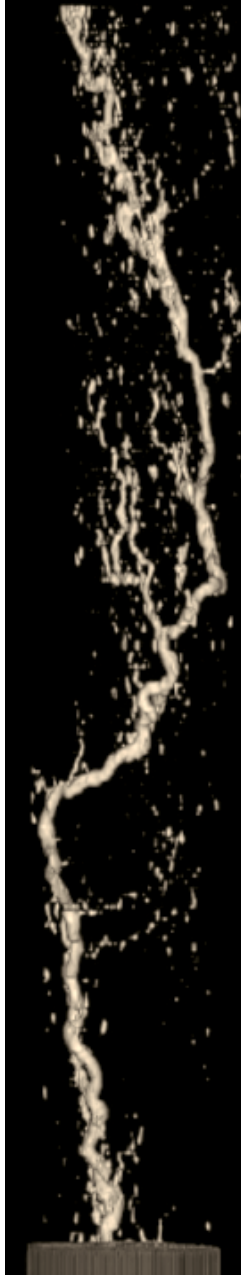
Figure A-67. CT Scan image of IC112: v_i = 1.92 cm/min, PV_{BT} = 0.49
