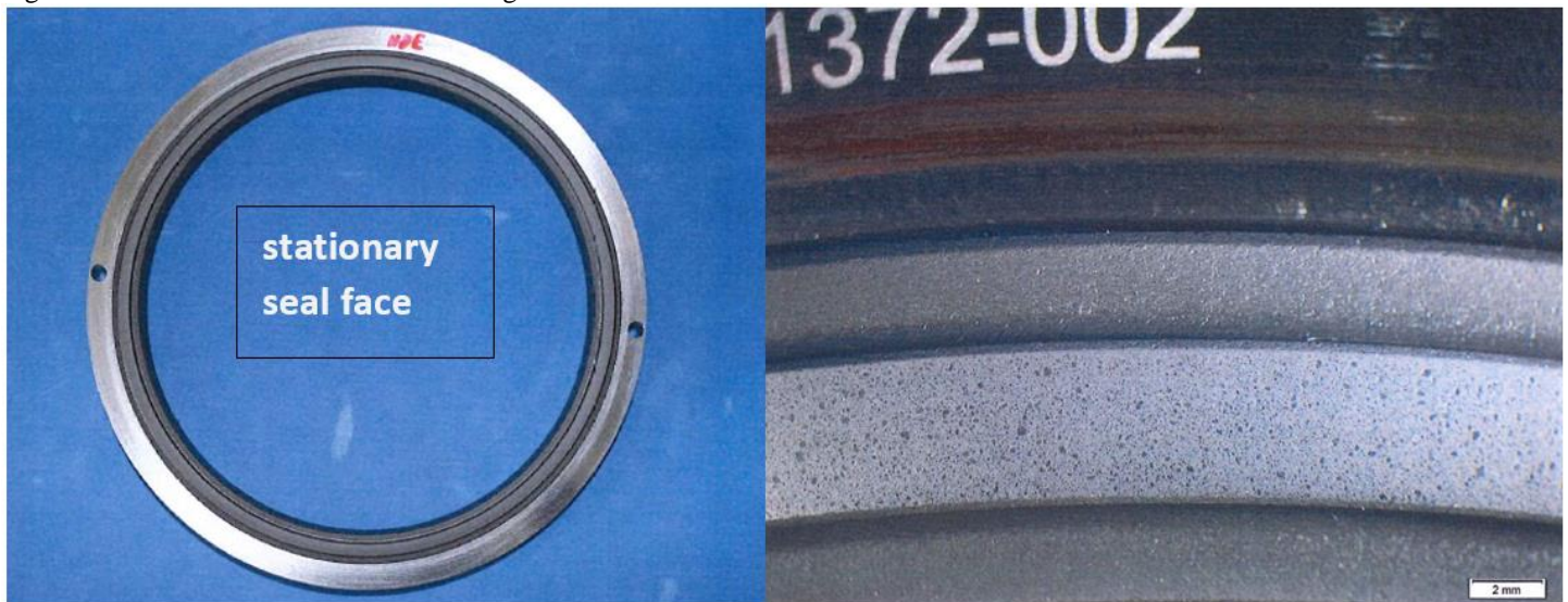
Figure 7: Seal face after 170 hours of testing
