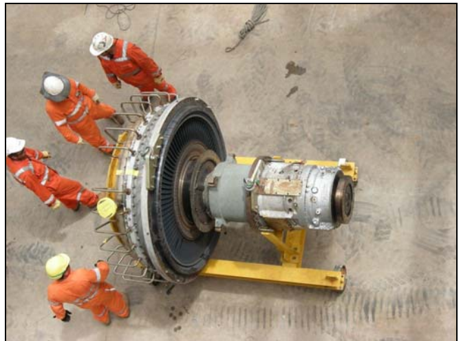
Figure 37. Power Turbine Module
