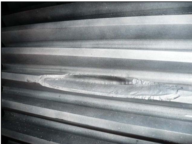
Figure 31. Gear Tooth Breakage.
