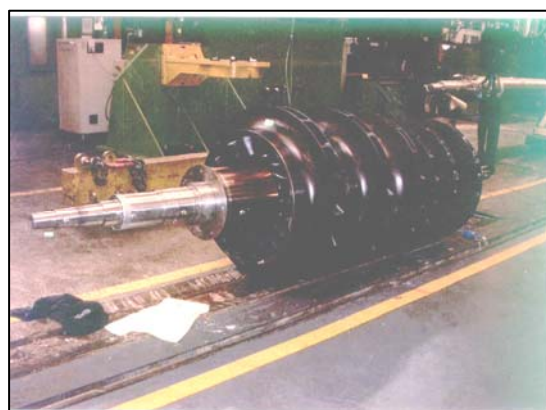
Figure 24. Ethylene Compressor Rotor with six Impellers in Back-to-Back Configuration.
