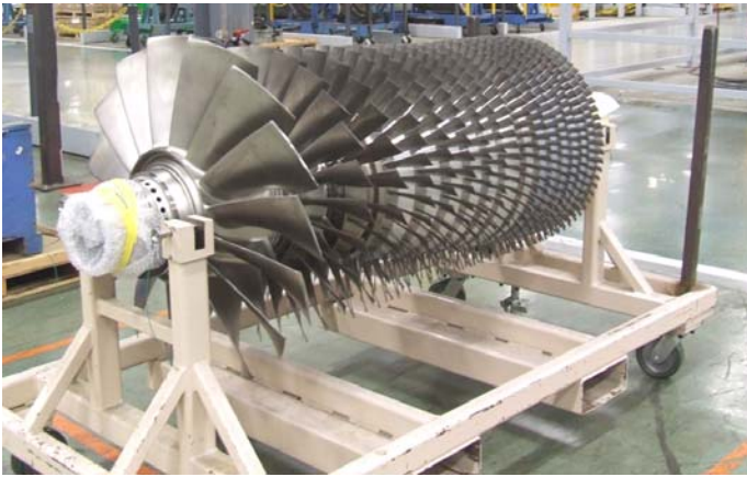
Figure 8. 17 stage Axial Flow Compressor of Gas Generator.
