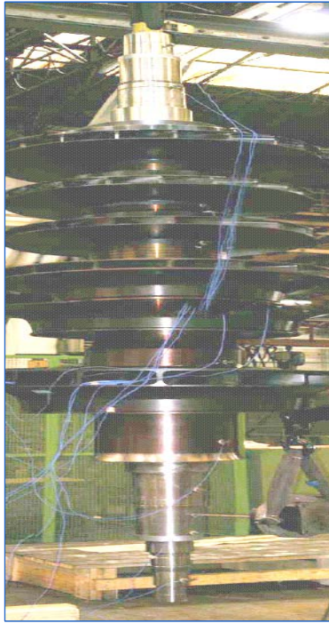
Figure 27. Free- Free Rotor Modal Testing
