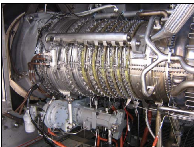
Figure 43. Gas Generator Showing Torque Tube for Variable Geometry Control.
