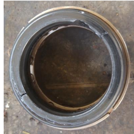
Shattered Rotary Seal Face
