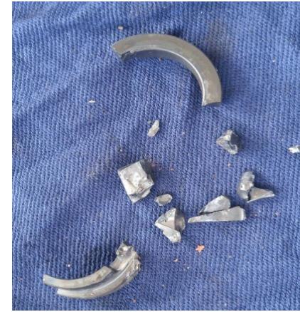
Shattered Stationary Seal Face
