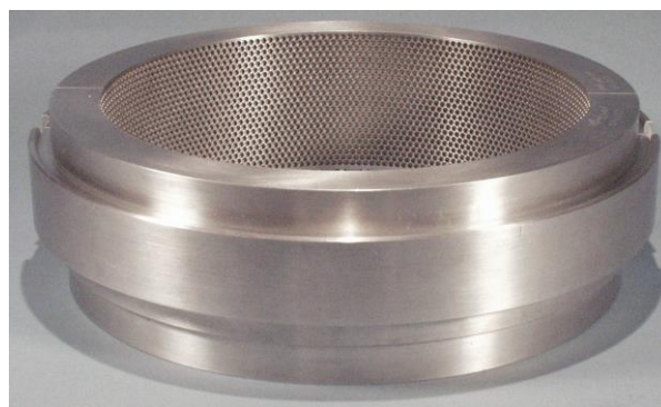
Figure 9: Example Hole Pattern Damper Seal (Moore et al., 2002)
