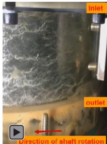
Fig. 8 Flow visualization of air-oil mixture, inlet GVF=0.9. Supply pressure 2 bara, discharge pressure 1 bara. Shaft speed 1.8 krpm. Videos at 60 frames/s taken with a stroboscope light with frequency = 30 Hz to freeze the shaft rotation motion. (Click here for Web (URL) Link).
