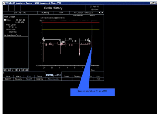
Figure 12: Vibration trip on 9 January, spiked up to 10g or more.
