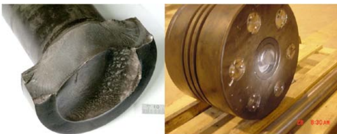
Figure 13: Piston rod failure.
