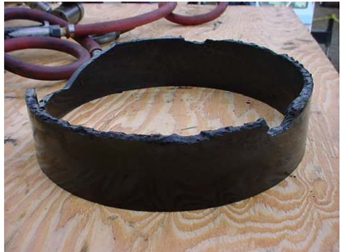
Figure 5: Rider band failure.
