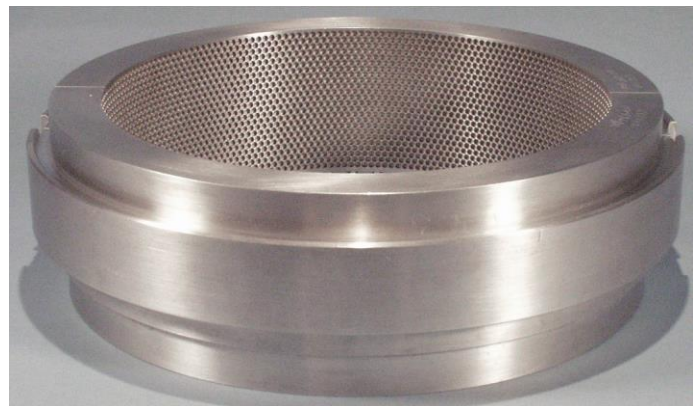
Figure 13: Example Hole Pattern Damper Seal (Moore et al., 2002)
