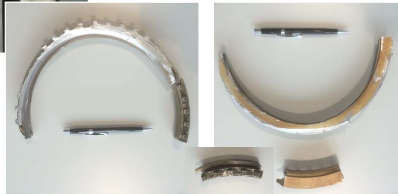
damaged diffuser vanes found in stages 3, 4 & 5 only
