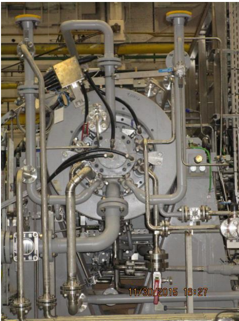
Figure 1: Gas lift centrifugal compressor with 4,500 psia (310 Bara) discharge pressure.
