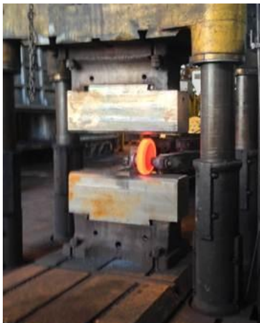
Figure 14 Experimental alloy melting and forging
