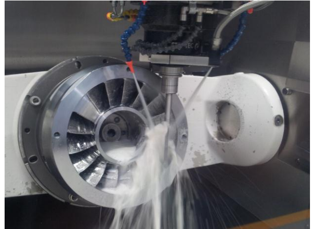
Figure 11 IN718 impeller under rough turning operation
