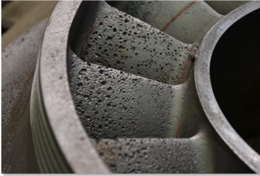
Figure 5 Heavy pitting on impeller flow path
