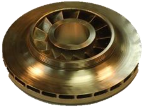
Figure 20 DMLM IN718 Impeller diam.120mm
