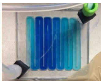
Fig. 4.3. A sample holder made by Lexan used for D - T_2 measurement. The s-patterned channels are 1.5 mm deep and across a 5 cm \times 5 cm area. The blue dye inside the channel was used to confirm an appropriate injection time for delivering the sample in the holder. No bubbles were observed after sample transport.
