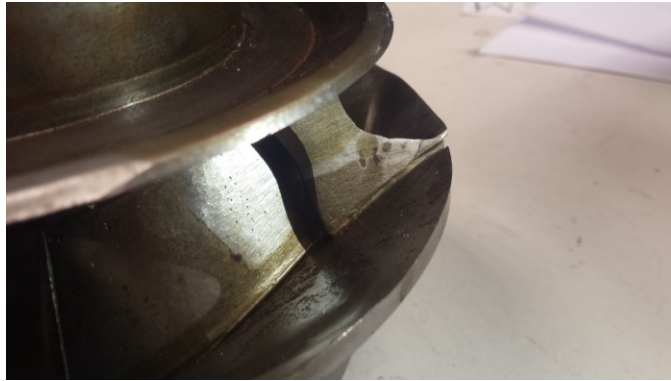
Figure 83. 1 st stage impeller blades after G400 20%GVF test
