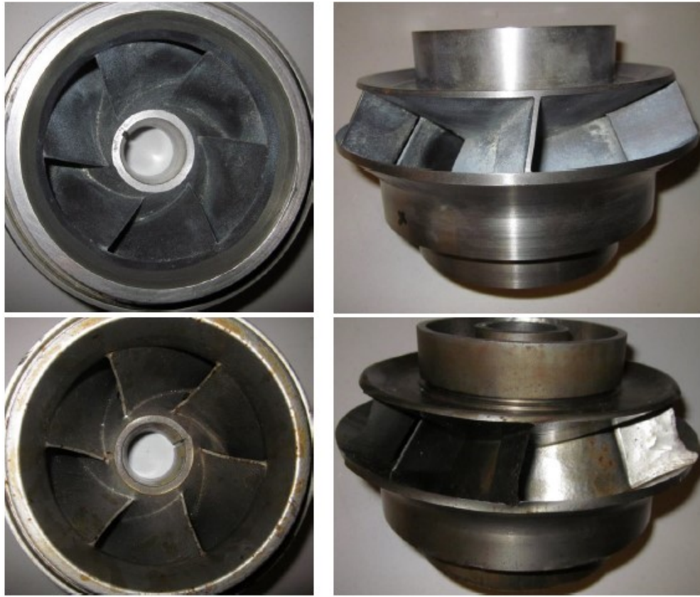
Figure 51. General view of 2 nd diffuser and impeller before and after test (Steck, 2014).
