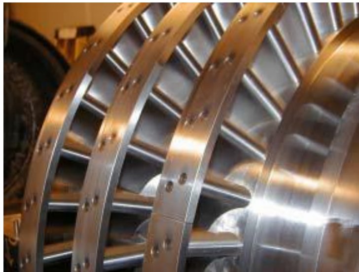
Figure 2. A three-stage high pressure research turbine at TPFL. The blades are cylindrical with tip shroud to reduce the tip leakage losses; Reprinted from Schobeiri [1].
