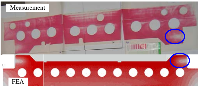
Figure 8. Pressure distribution after pretension (FEA and Film).
