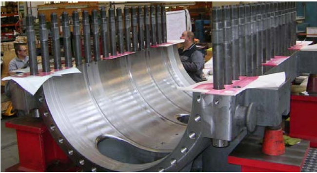
Figure 7. Opened casing with pressure films.
