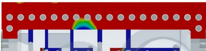
Figure 16. Gap distribution in the horizontal flange.
